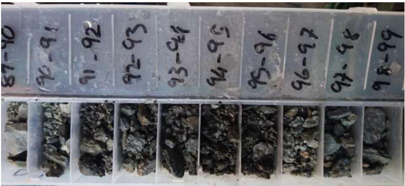
**Figure 1:** RC Drill chips from CMIPT031 showing massive sulphide from 91 to 98 m.
