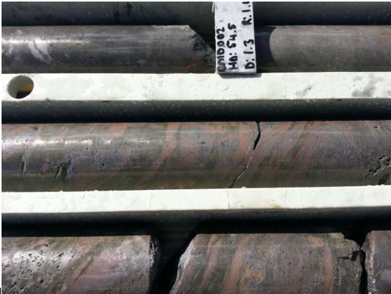
Figure 2. Massive pyrite (bronze-green colour), sphalerite (pale brown-pink) and galena (silver-grey) in CMD002 at Main Shaft.
