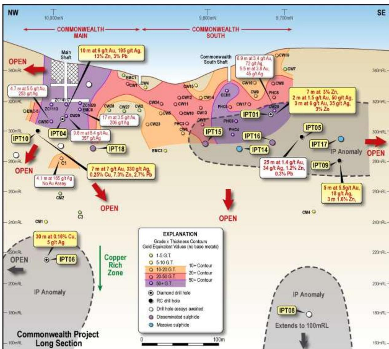
**Figure 1.** Long Section between Main Shaft and Commonwealth South Prospects showing the location of Impact's drill holes, previous drill holes, significant gold and silver mineralisation, IP anomalies and new drill intercepts in yellow boxes.
