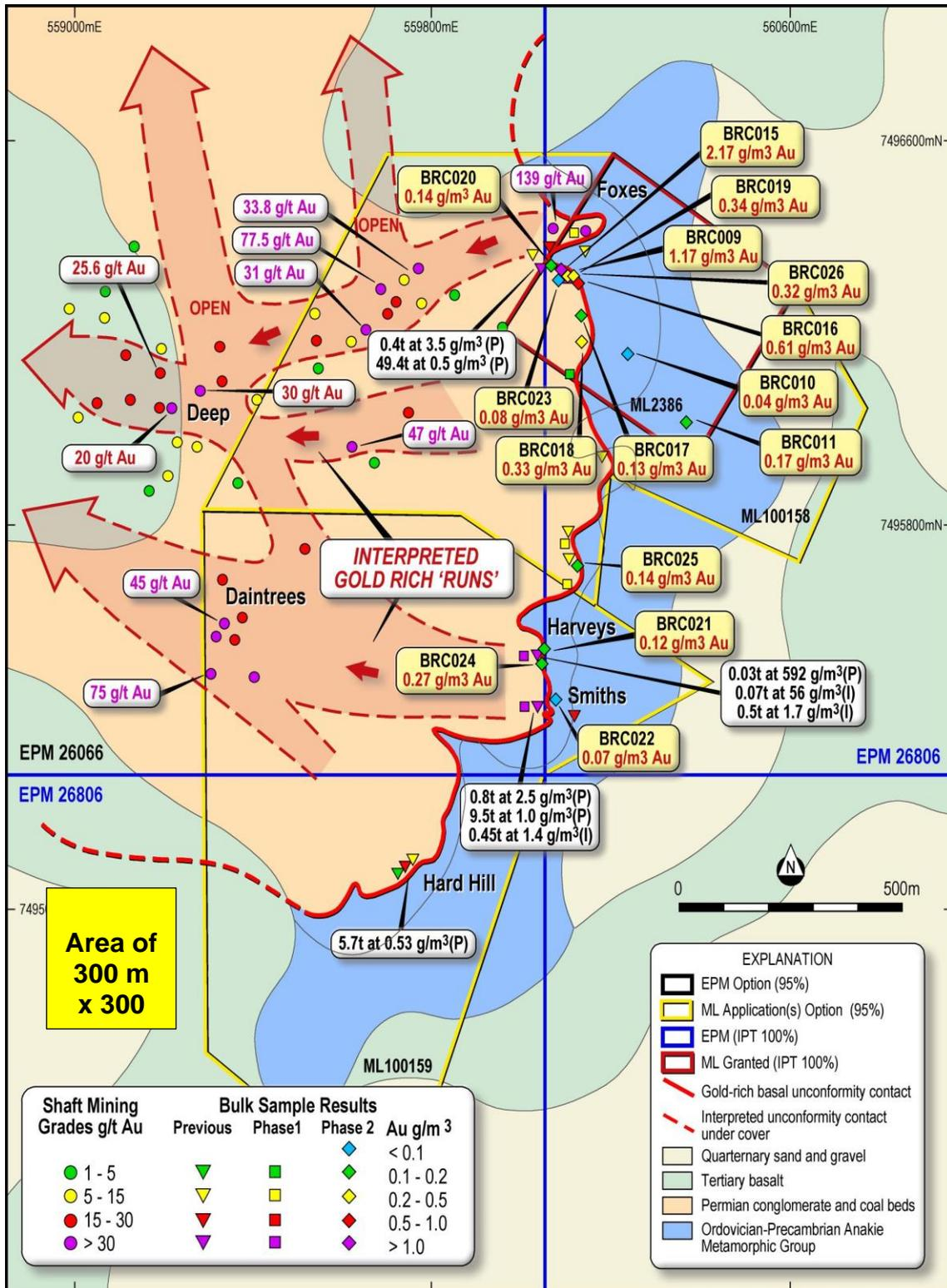
**Figure 1.** Gold results, previous gold production, geology and mining lease locations for the central Blackridge project area. All results are presented in grams per loose cubic metre. The second phase sample results are highlighted in the yellow call out boxes. An example of an area comprising 1,000,000 million cubic metres (310 m by 310 m by 10 m thick) is also shown for comparison.
