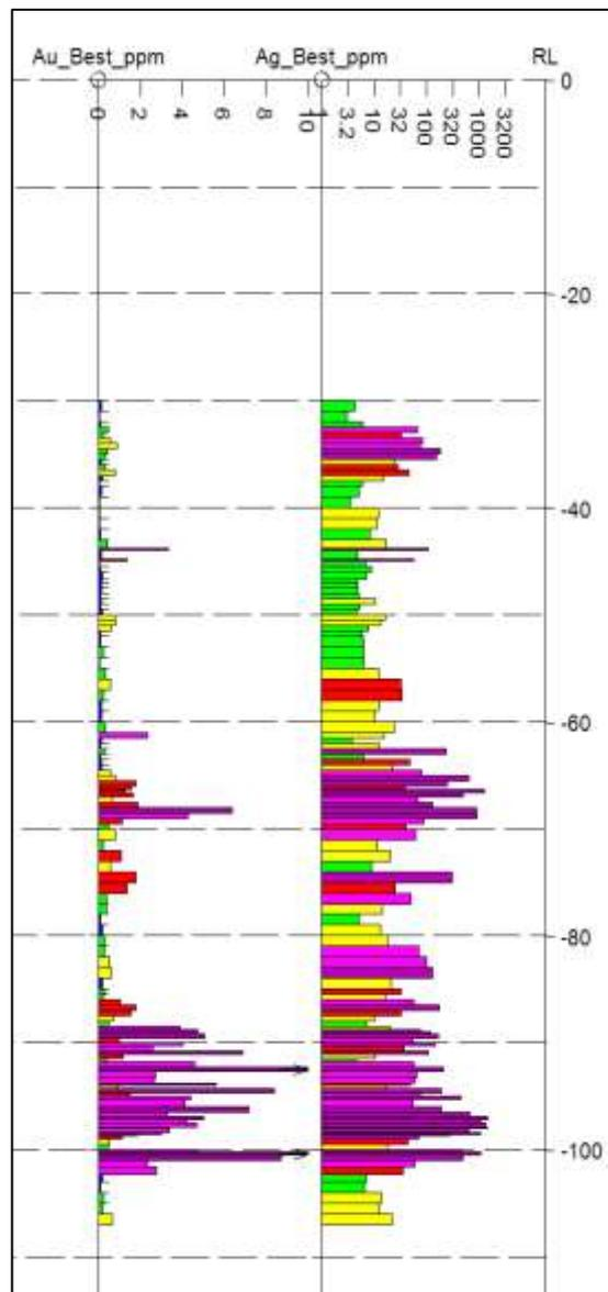
**Figure 4.** Detail of gold and silver assays for Hole CMIPT046. Note that the gold grades have been cut off at 10 g/t, and silver grades are at log scale to allow proper visualisation of the grades of up to 10 g/t gold and 1,490 g/t silver.
