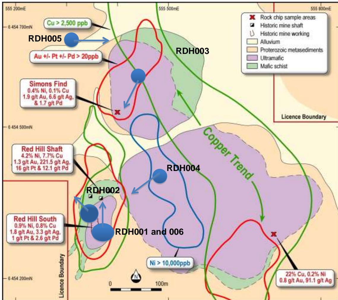
**Figure 3.** Geology of the Red Hill Prospect showing drill hole locations and soil geochemistry results and rock chip assays.
