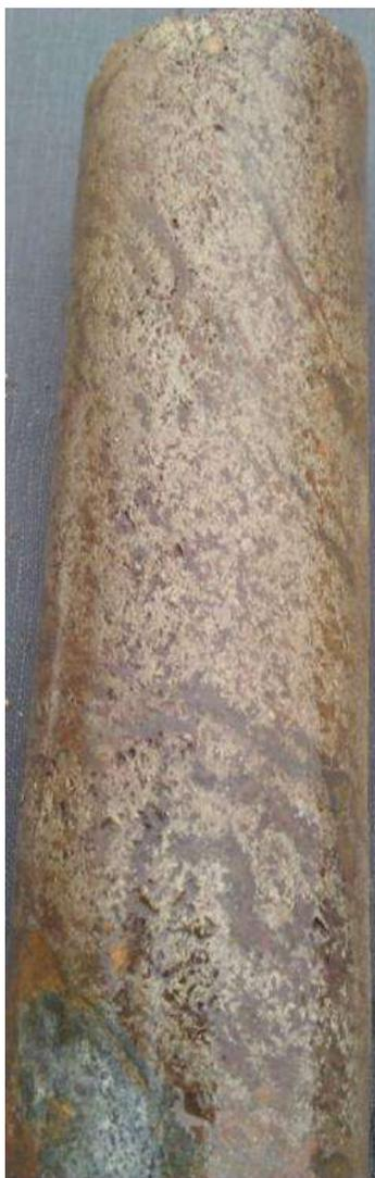
**Figure 1.** Massive sulphide with nickel and copper from 58 m
