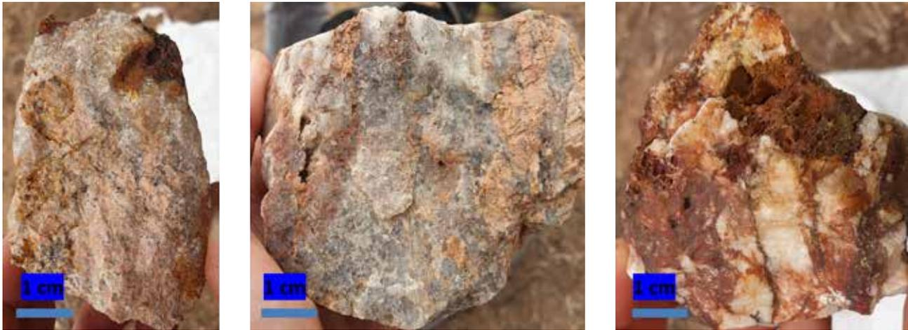
**Figure 9:** Gradation of veins from K-feldspar dominant (left photo) to quartz-dominant (right photo) with increasing boxwork gossan (dark brown colour) from weathered sulphides.
