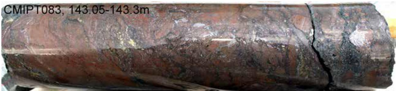
**Figure 13:** Second massive sulphide unit in Hole CMIPT083: massive and brecciated massive sphalerite (red-brown) with lesser galena. Up to 3% chalcopyrite (yellow) is present in places.
