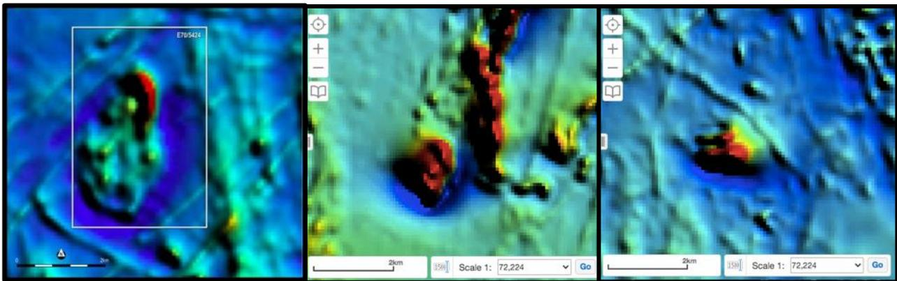
**Figure 11.** Image of regional magnetic data showing the magnetic anomalies at Beau (left), Gonneville (Chalice Mining Ltd centre) and Newleyine (right) for comparison.
