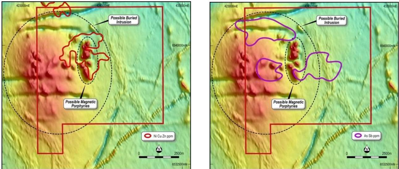
**Figure 15.** Images of the regional magnetic data showing a nickel+copper+zinc anomaly over the shallow magnetic anomalies (left) and an outer halo of arsenic+antimony (see ASX Release 17<sup>th</sup> November 2020 for details on the soil geochemistry anomalies).
