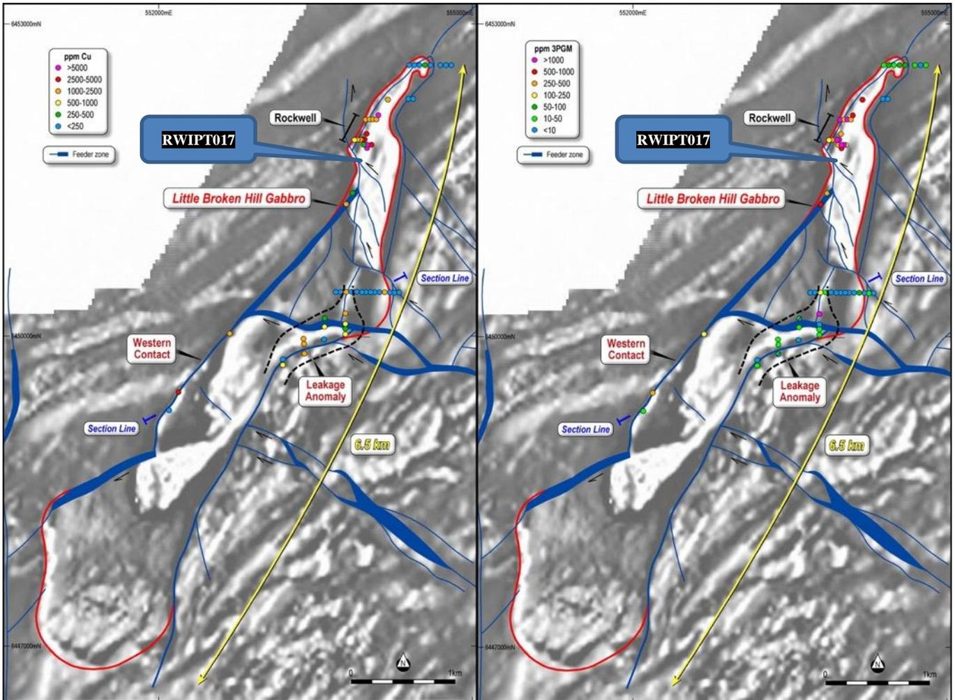
**Figure 2.** First vertical derivative image of airborne magnetic data over the Little Broken Hill Gabbro showing interpreted feeder zones in blue, Impact’s drill collars and best results down hole for copper and 3PGM (palladium+platinum+gold). Note the widespread mineralisation over the length of the intrusion. The LBHG is clearly very fertile with significant potential to discover a major PGE-nickel-copper deposit.
