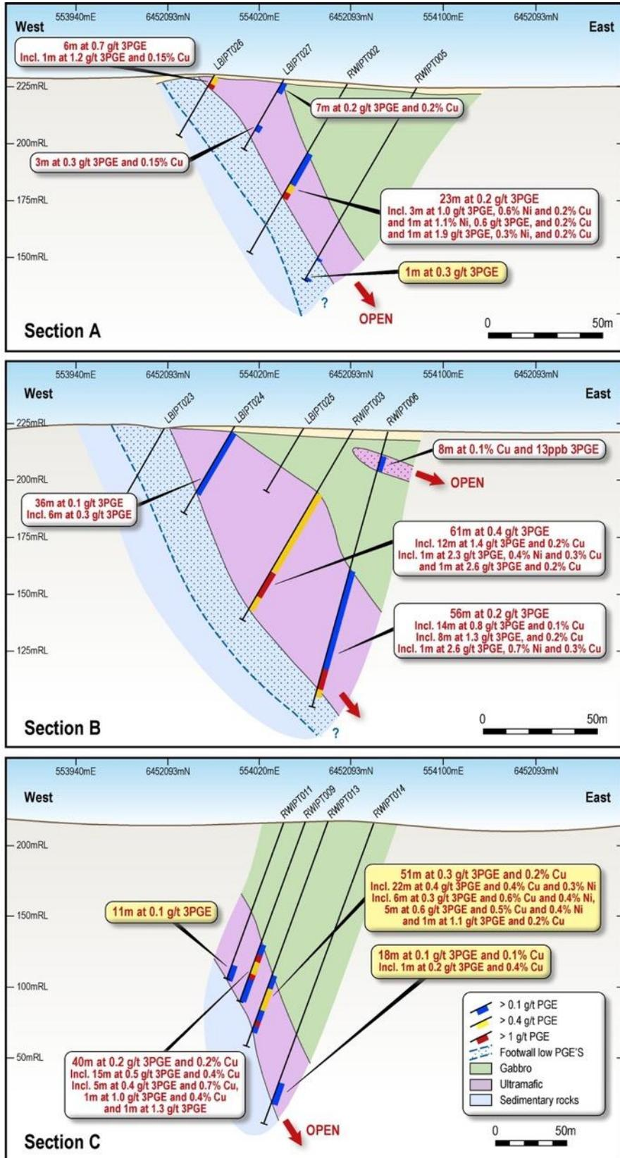
**Figure 3.** Cross-sections through the Rockwell Prospect with recent drill results in yellow. Note the increasing PGE content with width of the basal ultramafic (see Figure 4 for location of cross sections from Drill Hole IDs).
