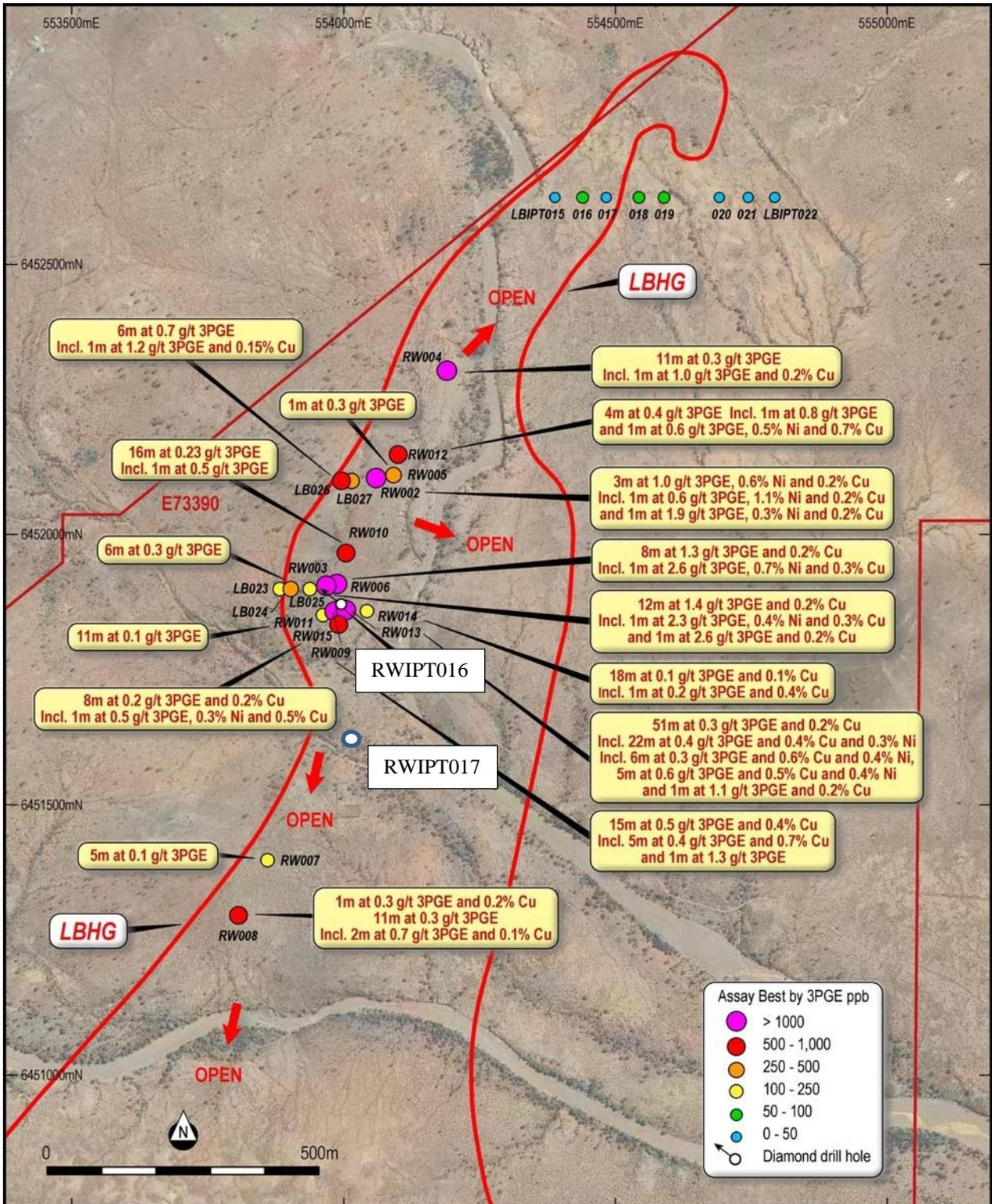
**Figure 4.** Location of Impact’s drill holes at Rockwell with best down hole assay results for 3PGE and showing the location of diamond drill holes RWIPT016 and RWIPT017 (ASX Release 23<sup>rd</sup> June 2021). The northern line of drill holes with weaker results are vertical aircore drill holes that are no more than 50 metres deep. They have probably not effectively tested the basal ultramafic unit at depth and deeper RC drilling is required.
