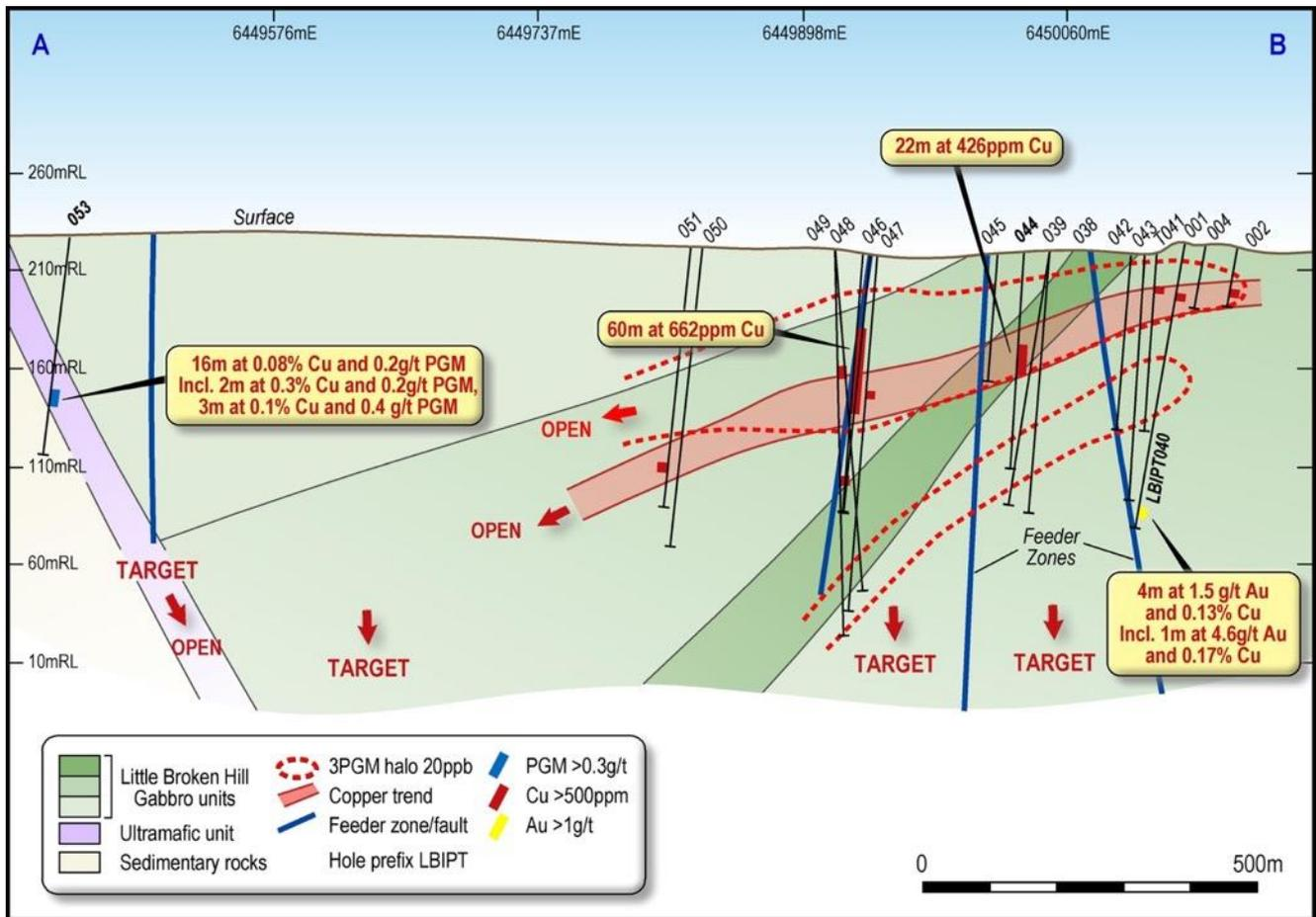
**Figure 7.** Oblique cross section through the LBHG showing drill results from the Central LBHG area and also the Western Contact (Hole 053). Significant anomalous copper and 3PGE mineralisation is present over a large area and at depth. This is encouraging for the discovery of a massive sulphide deposit at depth.
