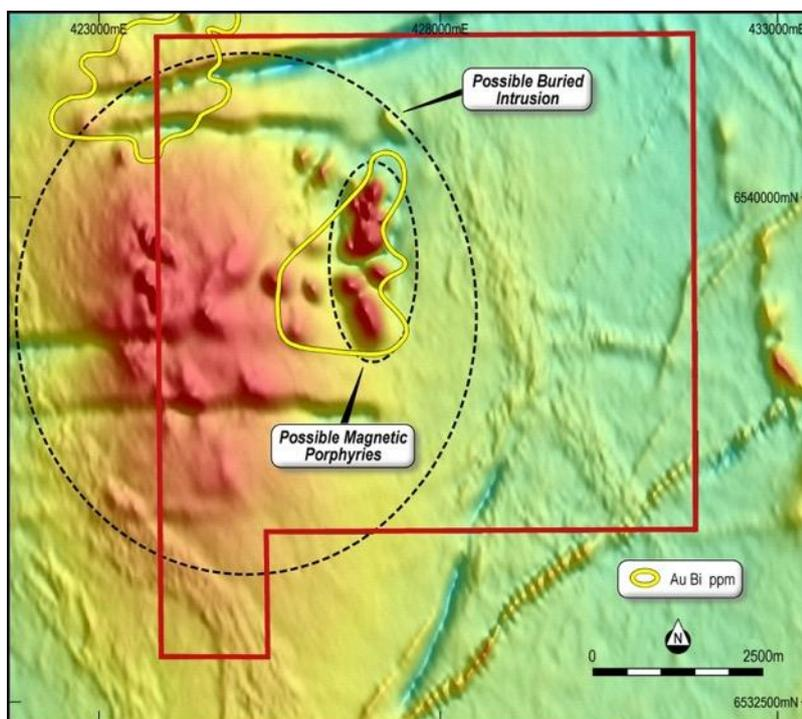
**Figure 14.** Image of regional magnetic data over the Doonia project with warmer colours indicating more magnetic units. A large oval deep-seated anomaly is centred directly under the project area above which a cluster of near surface anomalies is present and which are interpreted as possible magnetic intrusions. These smaller anomalies are coincident with a gold-bismuth soil geochemistry anomaly (ASX Release 17<sup>th</sup> November 2020).
