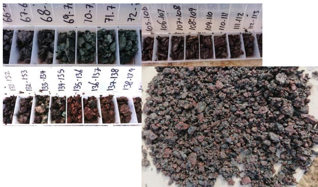
**Figure 8.** Alteration in Hole APIPT001. Strong chlorite-epidote alteration (top left) passes into strong hematite alteration (top right) then strong K-feldspar alteration in a porphyritic unit (bottom left). A close up of the strong K-feldspar unit is shown in the bottom right from 137 metres downhole and is typical of more proximal alteration.
