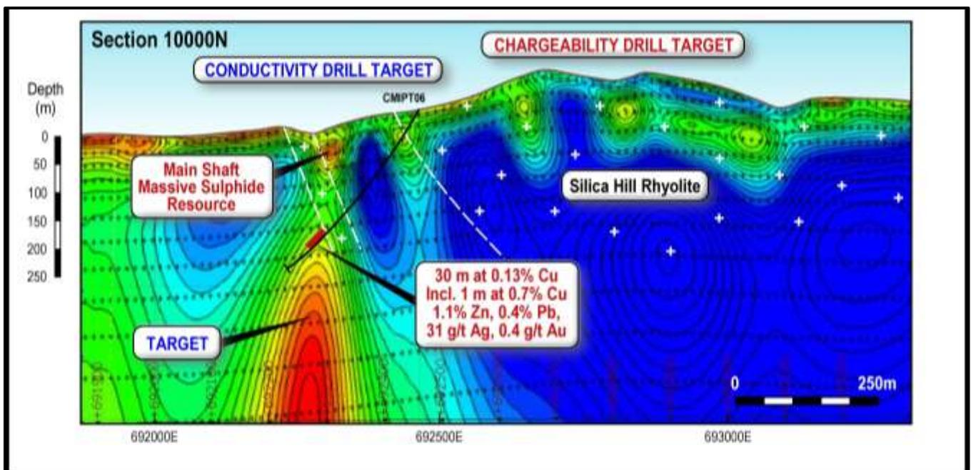
**Figure 2.** IP Conductivity data along Section 10,000 mN showing the massive sulphide body at Main Shaft and copper-rich drill hole CMIPT06.
