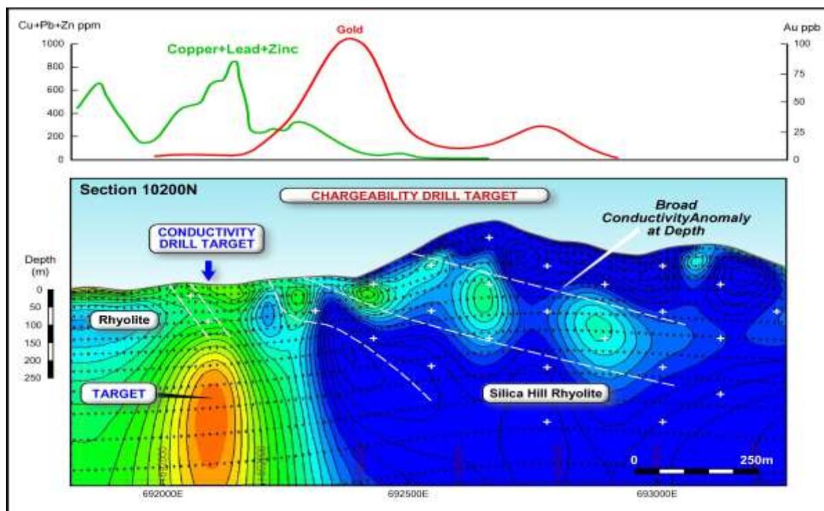
**Figure 3.** IP Conductivity data along Section 10,200 mN showing coincident IP conductivity and lead-zinc-copper-in-soil anomalies. The gold-in-soil anomaly is coincident with strong IP chargeability anomalies (see announcement [9 May 2017](#)).
