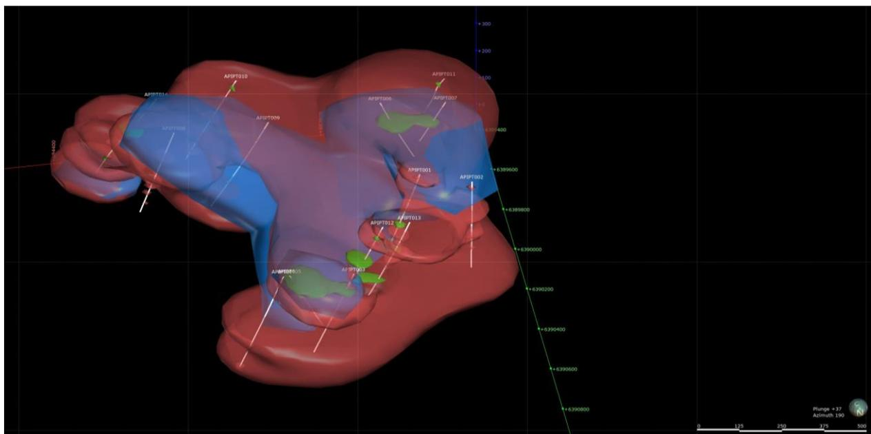
**Figure 1.** View looking South of the copper halo (red bubbles >100 ppm copper, green bubbles >200 ppm copper) with an associated molybdenum halo (>2 ppm molybdenum). Thick intercepts of low to modest grade copper occur over an area of at least about one square kilometre.
