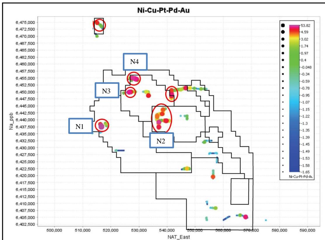
**Figure 5.** Additive Z scores for Ni-Cu-Pd-Pt-Au across the main Arkun project area. Note the large areas of anomalism in the central part of the project area. Six priority areas for follow up work are highlighted. Other areas of elevated response are also evident including the Beau target to the north.
