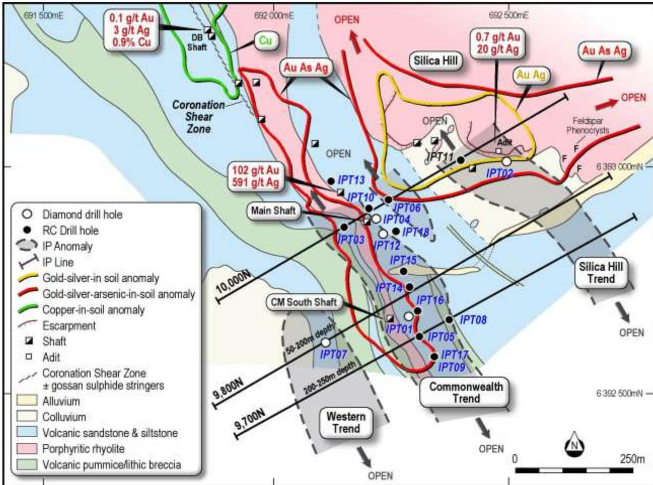
**Figure 3.** Geology of the Commonwealth area showing drill holes completed so far and the location of the IP Survey Lines and soil geochemistry results.
