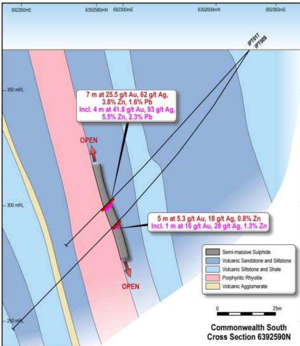
**Figure 2.** Cross section on 6,392,590 mN showing the location of the new massive and semi-massive sulphide layer at the top of the host rhyolite unit. Note that the massive sulphide includes extensive pyrite as well as sphalerite, galena and lesser chalcopyrite.
