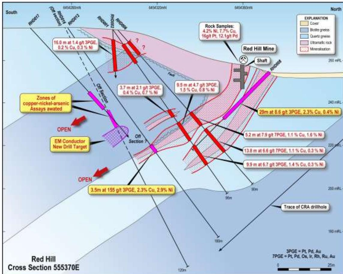
Figure 1. Cross section through the Red Hill Prospect.
