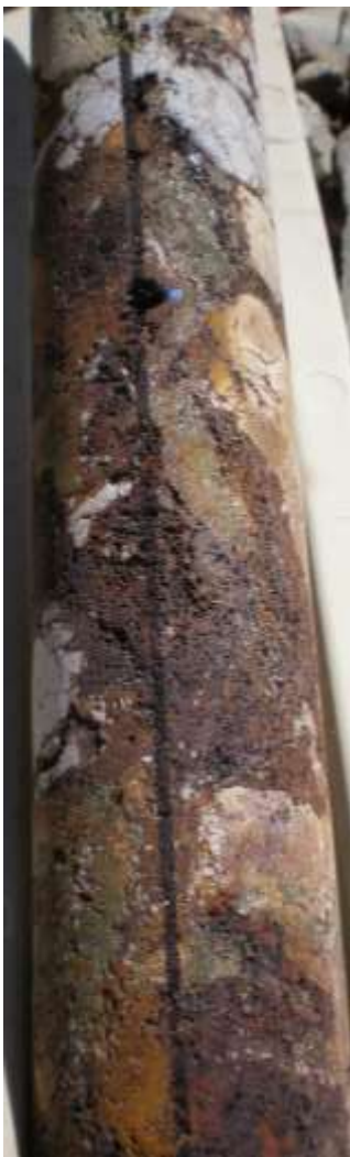
Figure 2a. Boxwork gossan texture replacing massive iron sulphide and containing up to 1.1% nickel and 3.3% copper by XRF.
