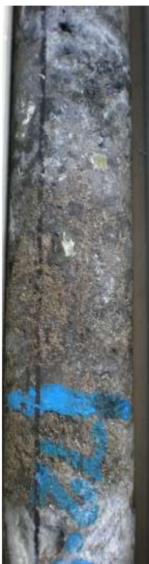
Figure 1. Nickel and iron sulphides with up to 5.3% nickel (by XRF).
