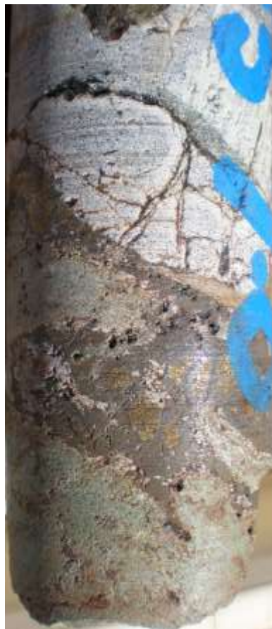
Figure 2b. Iron oxide (haematite) replacing iron sulphide and nickel sulphide with fresh copper sulphide in vein at contact between metasediment and thin mafic unit. XRF assays up to 8.3% nickel and 5.6% copper.
