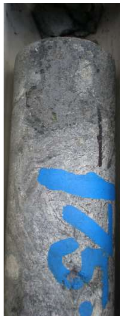
Figure 2c. Contact between metasedimentary rock and 15 cm thick chalcopyrite-chalcocite (secondary sulphide) XRF assays up to 20% copper.
