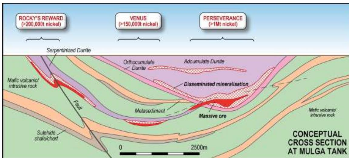
Figure 3. Conceptual cross-section for the Mulga Tank Dunite and surrounding area showing the Perseverance and Rocky's Reward exploration model.
