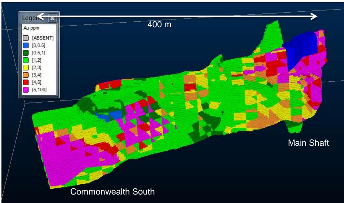
Figure 2. Block model of the resource from Commonwealth South (left) to Main Shaft (right). The distribution of the high grade blocks in pink show that the deposit is open along trend and at depth.
