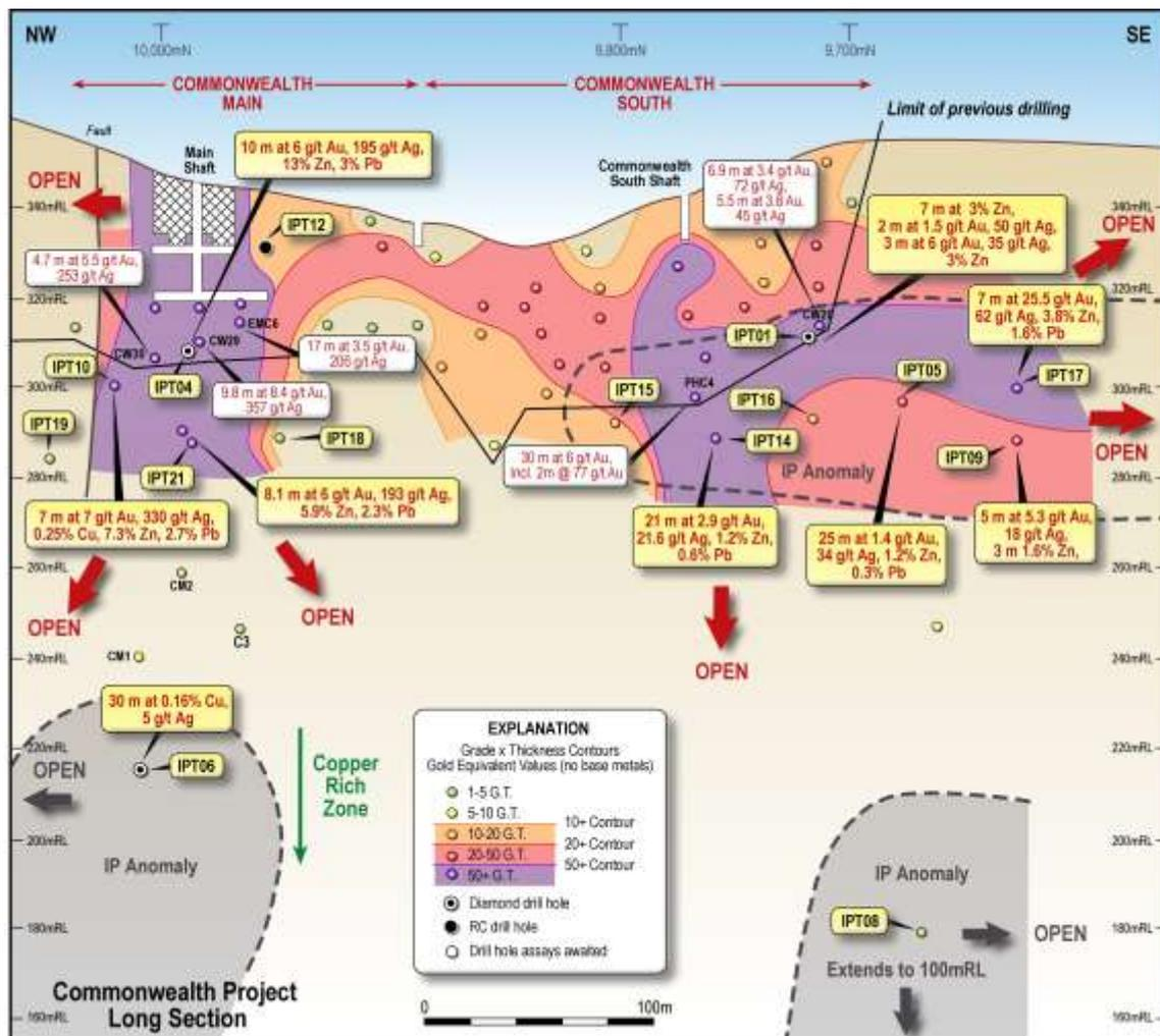
**Figure 3.** Long Section between Main Shaft and Commonwealth South Prospects showing drill hole locations, gold and silver mineralisation, IP anomalies and Impact’s drill intercepts in yellow boxes.
