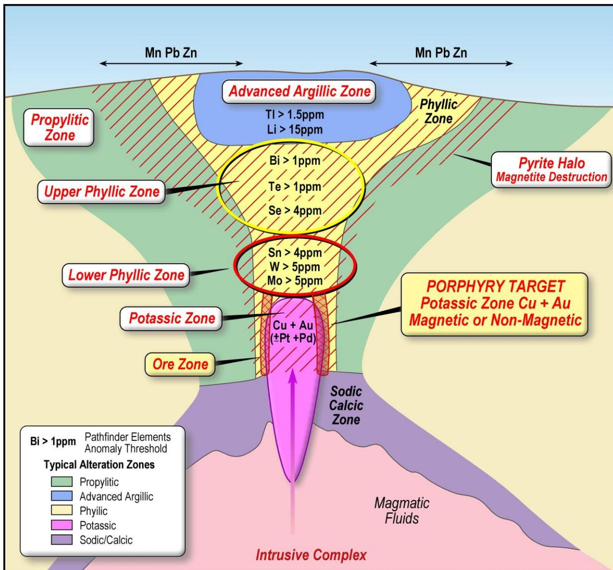
**Figure 7.** Model of the alteration zones and metal assemblages expected around major porphyry copper-gold deposits. In plan view these zones would be concentrically arranged around the host porphyry and this gives rise to the zinc doughnut phenomenon as shown for Wafi-Golpu shown below. Here soil geochemistry data for zinc shows a well developed annulus around the centre of the porphyry copper-gold deposit. Note the scale of the system which is similar to that defined at Apsley.
