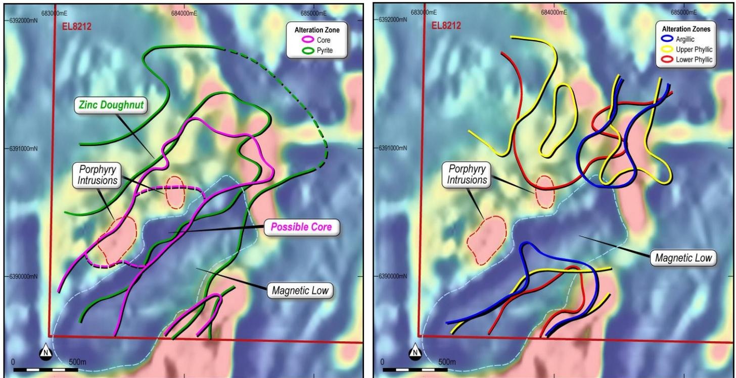
**Figure 5.** Image of the airborne magnetic data with more magnetic units in warmer colours and highlighting the possible parent porphyry intrusions and significant magnetic low.
