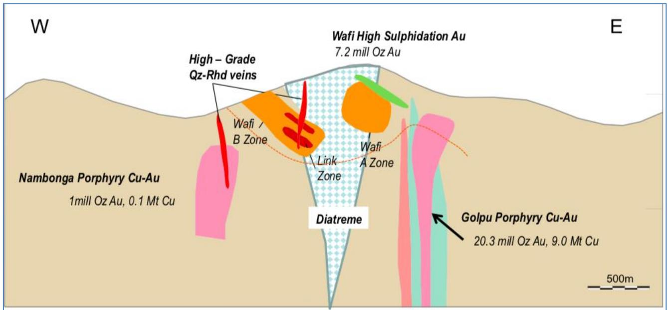
**Figure 6.** Schematic cross-section across the Wafi-Golpu porphyry-copper gold system and related epithermal gold veins. Note there are several porphyry intrusions within an area of about 2 to 3 square kilometres.
