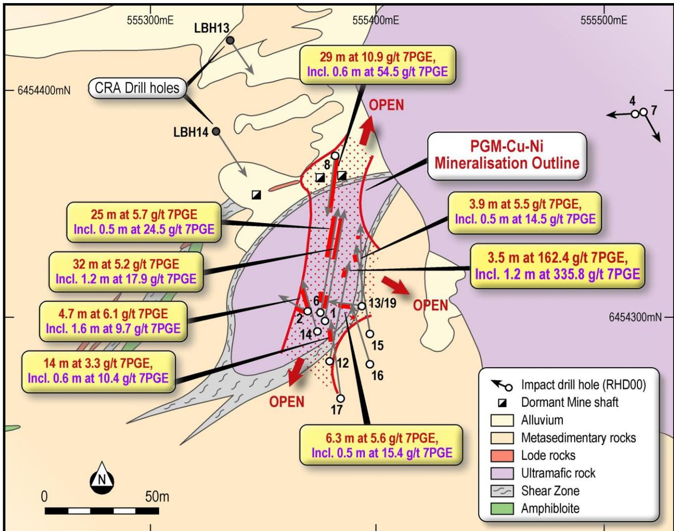
**Figure 2.** Drill hole location plan for Red Hill showing the location of the recently reported assay results (see ASX Release 7<sup>th</sup> May 2020 for details).
