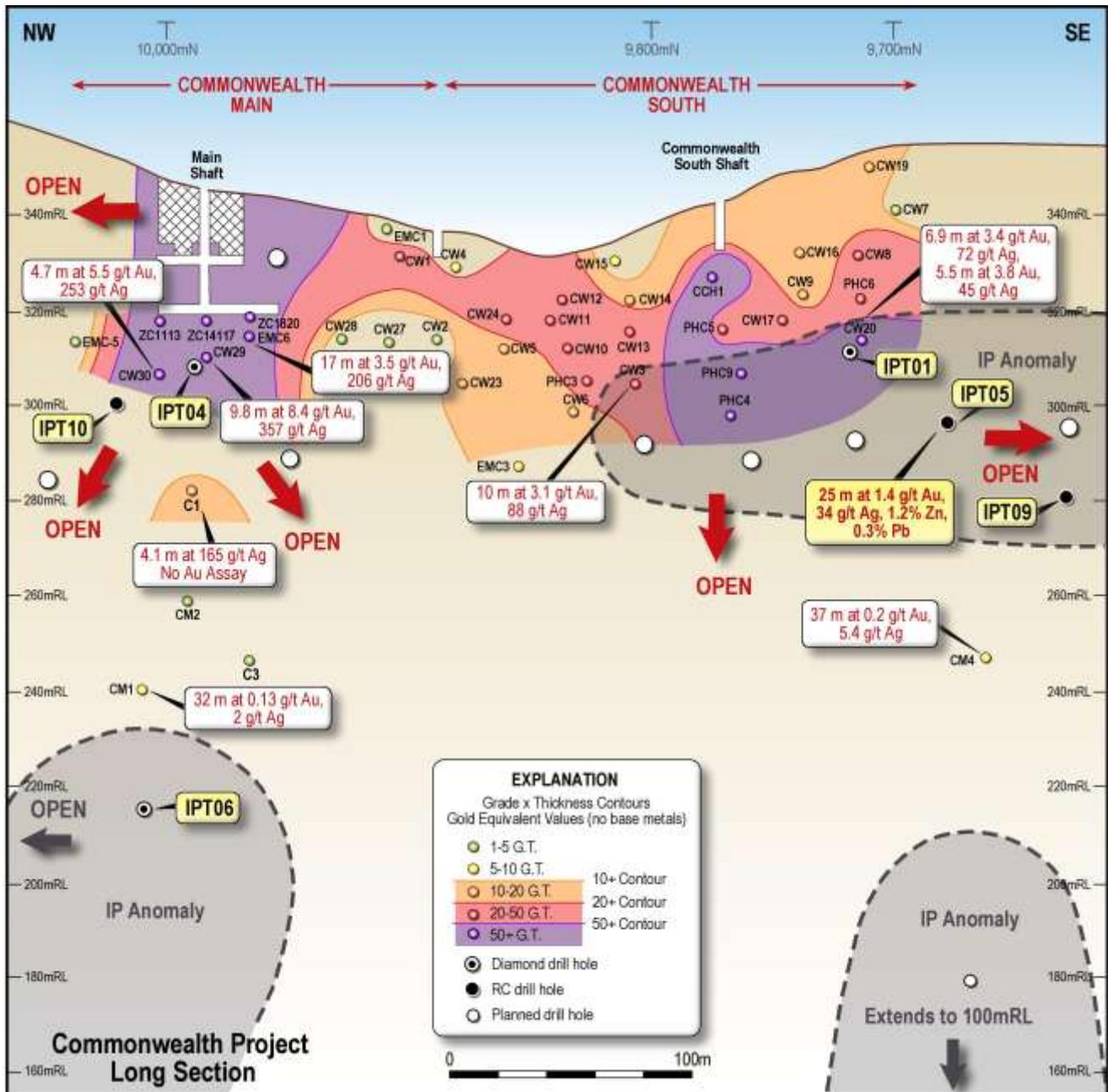
**Figure 1.** Long Section between Main Shaft and Commonwealth South Prospects showing the location of Impact’s drill holes, previous drill holes, significant gold and silver mineralisation and the IP anomalies.
