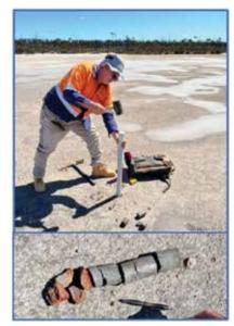
**Figure 4.** Lake Hope showing the push tube sampling method used to drill out the resource and an example of the lake clay from the push tube.
