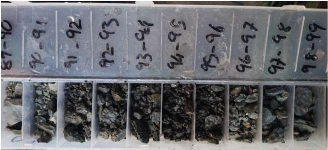
**Figure 1:** RC Drill chips from CMIPT031 showing massive sulphide from 91 to 98 m.
