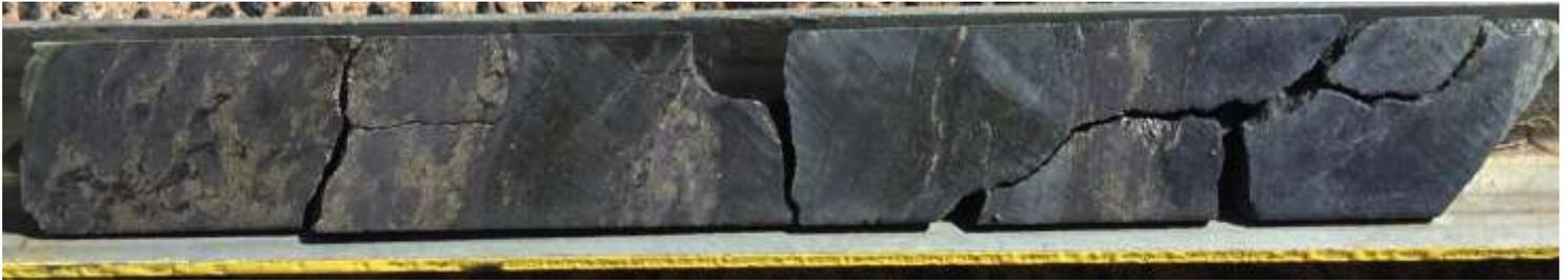
**Diamond drill core from Hole CMIPT011 showing semi-massive sulphide from a 0.9 metre thick zone that has returned 3,146 g/t or 101 ounces of silver and 2.4 g/t gold.**
