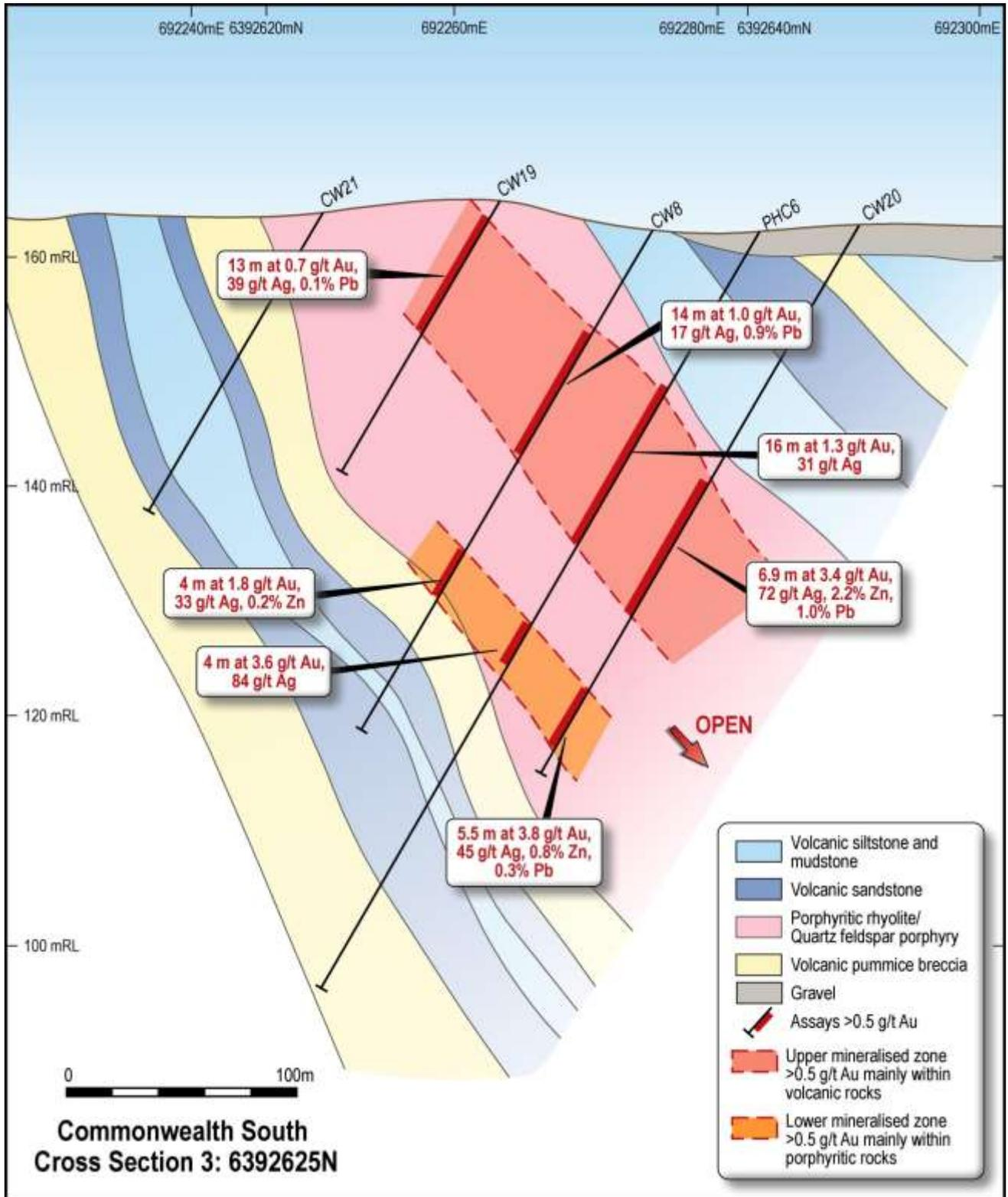
Figure 7. Cross Section 3 (Figure 4) showing the geology and key drill results at the southern end of the Commonwealth South Prospect.
