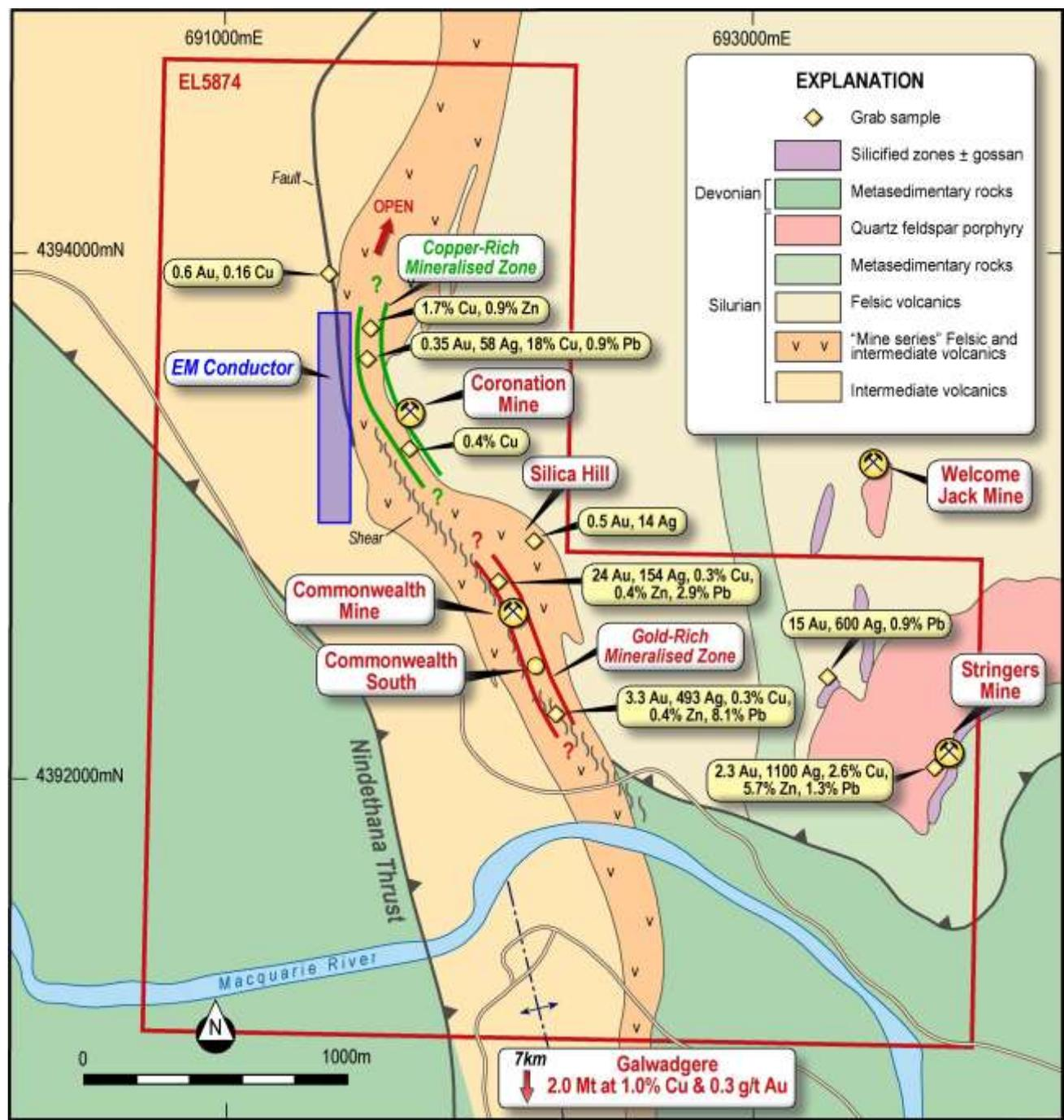
**Figure 3.** Commonwealth Project: Geology, Prospects and Significant Rock Chip Assays. Previous exploration focused solely only on 300 m of strike between the Commonwealth Mine and Commonwealth South Prospect.
