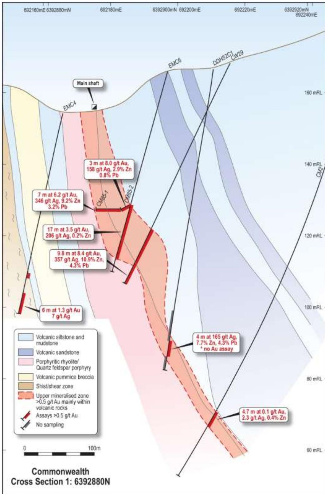
**Figure 5.** Cross section 1 (Figure 4) showing the geology and key drill results beneath the main shaft at Commonwealth.
