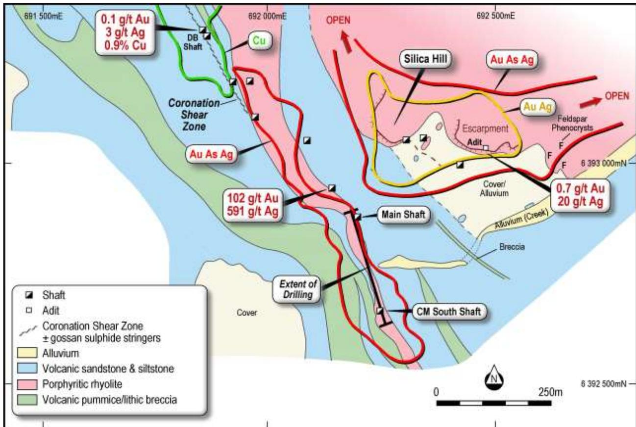
**Figure 1.** Geology and Soil and Rock Chip Results from the Commonwealth-Silica Hill area
