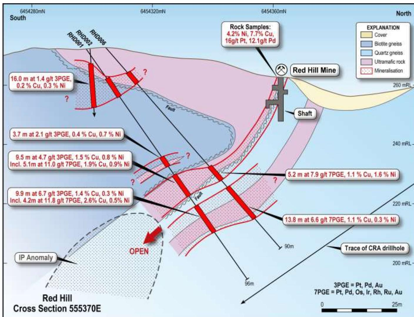
Figure 1. Cross section at the Red Hill Mine (see Figure 2 for location). Note that CRA Exploration completed two diamond drill holes under Red Hill in 1969 with no significant results. It appears these holes were drilled parallel to and below the mineralised zone.
