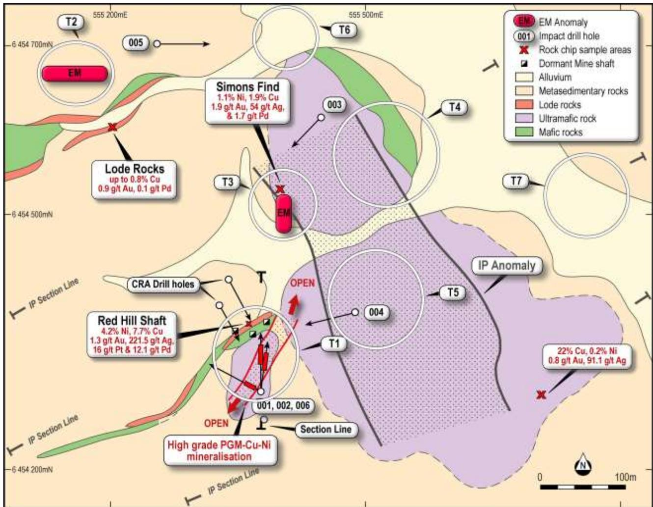
Figure 2. Geology and drill targets (white circles T1 to T7) at the Red Hill Prospect.
