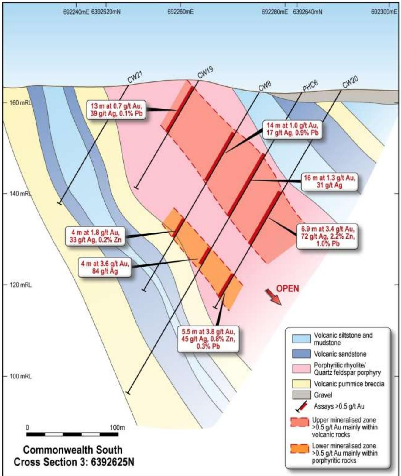
Figure 8. Cross Section 3 (Figure 5) showing the geology and key drill results at the southern end of the Commonwealth South Prospect.
