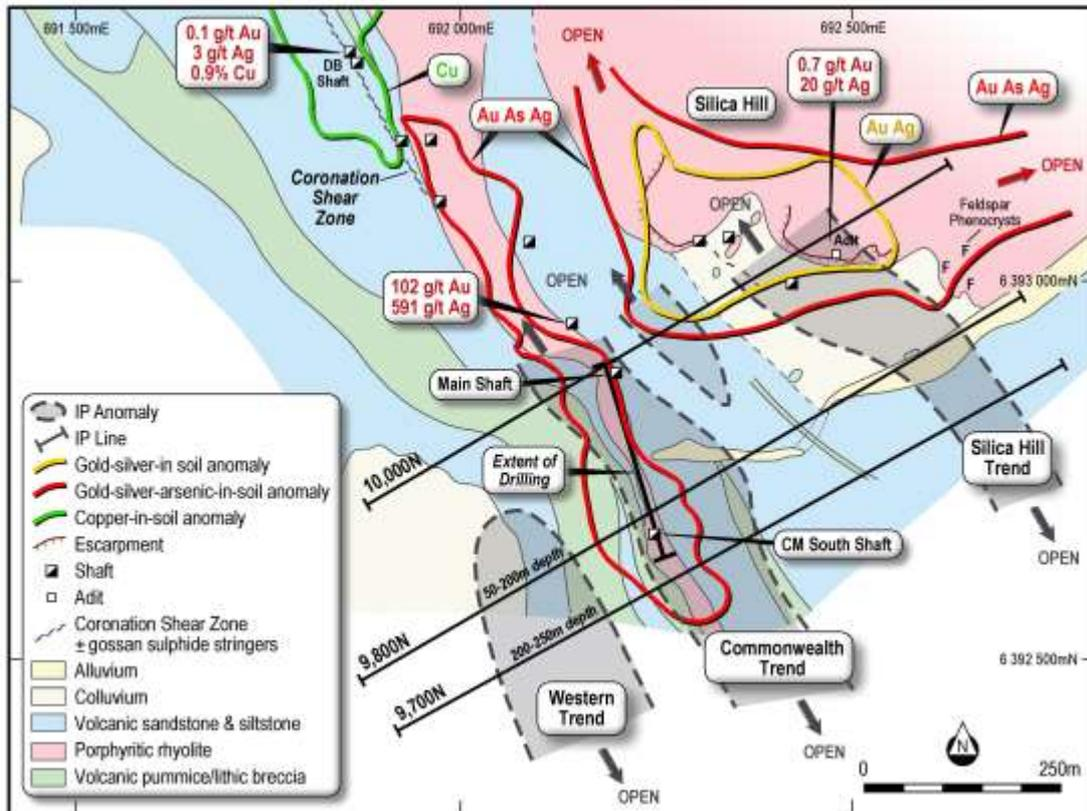
Figure 1. Geology of the Commonwealth area showing the location of the IP Survey Lines and soil geochemistry results (see announcement dated 12th May 2014).
