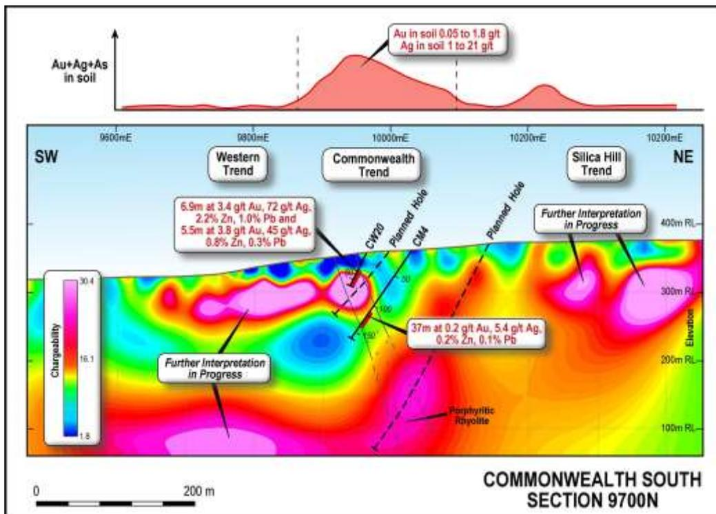
Figure 2. Results of an Induced Polarisation Survey over the Commonwealth South Prospect showing the three IP Trends and soil geochemistry responses over the areas. The Western Trend lies beneath alluvial cover (see Figure 1 for location of survey line).
