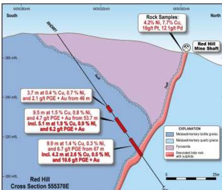
3. 3.7 m at 0.4% copper, 0.7% nickel, 2.1 g/t Pt-Pd-Au and 3 g/t silver from 46 m.
