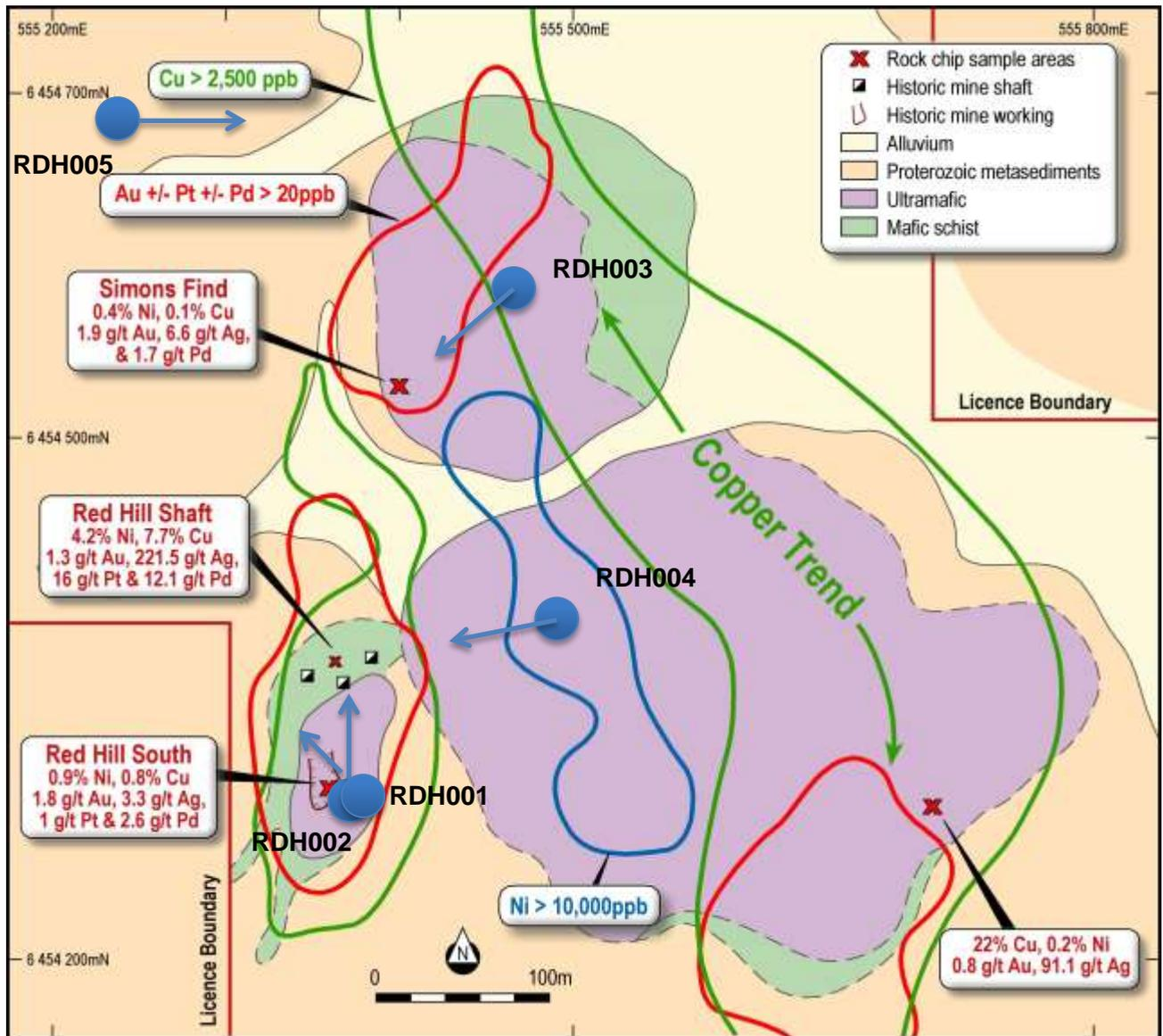
Figure 2. Geology of the Red Hill Prospect showing drill hole locations and soil geochemistry results and rock chip assays.
