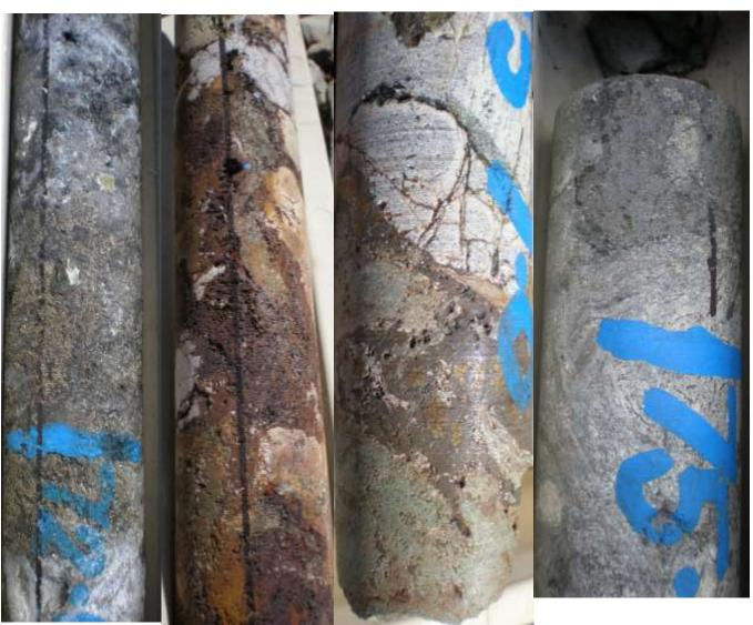
Figure 2a. Nickel and iron sulphides.
