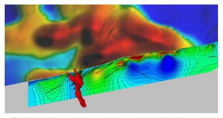
**Figure 8.** Three dimensional view from the south of the southern most IP line and showing the Commonwealth resource and the drill traces at Silica Hill with an image of silver-in-soil (red areas greater than 1 g/t silver) to the north of the IP line. There is an extensive undrilled silver-in-soil anomaly covering many hundreds of square metres.
