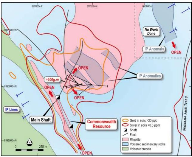
**Figure 2.** Silica Hill-Commonwealth area: Geology and exploration results. Drill traces shown for Silica Hill only to demonstrate the small area only partly tested to date. Note the area of greater than 100 gram.metre intercepts and the large untested coincident gold- and silver-in soil and interpreted IP chargeability anomaly trends. Note also the significant IP anomaly to the north east along the extension of the Welcome Jack Trend.
