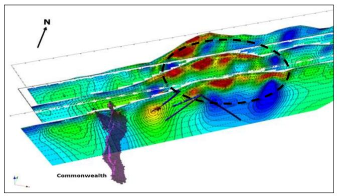
**Figure 5.** Three dimensional view from the south of the new IP data showing the extent of the chargeability anomalies (red areas win dashed oval) north of Silica Hill (drill traces shown in black) and also the location of the Commonwealth resource. The survey lines are 100 metres apart.
