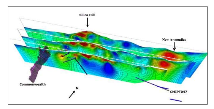
**Figure 7.** View of the new IP data from the south west showing the strong chargeability anomalies to the east of Silica Hill and to the north of Welcome Jack. No work has been done here.
