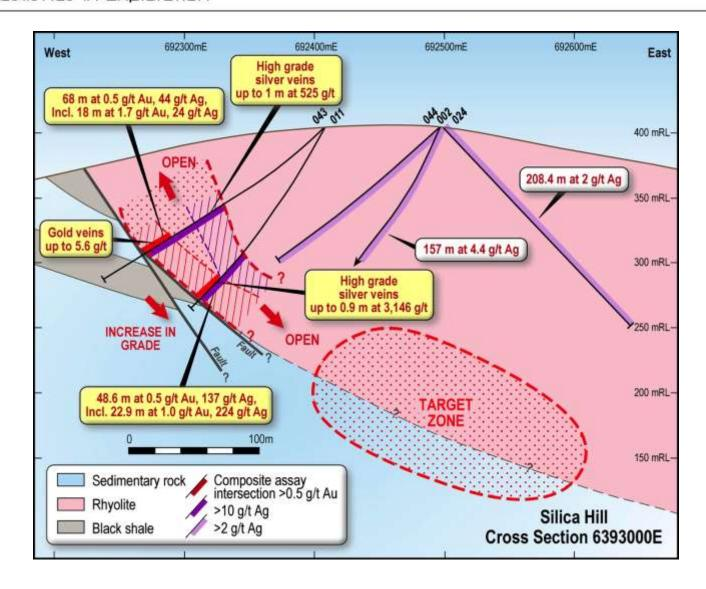
**Figure 9.** East-West cross section showing results for Holes CMIPT043 and 011.
