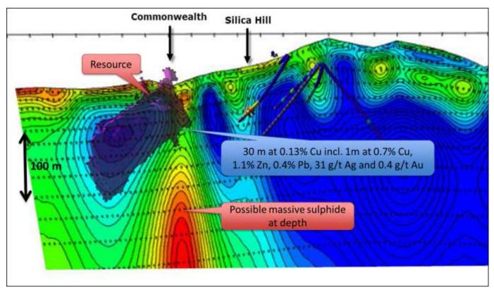
**Figure 6.** Three dimensional view looking north showing an image of the IP resistivity data with conductive zones shown in red and also showing the outline of the Commonwealth resource. Note the conductor at depth below the resource that is undrilled.
