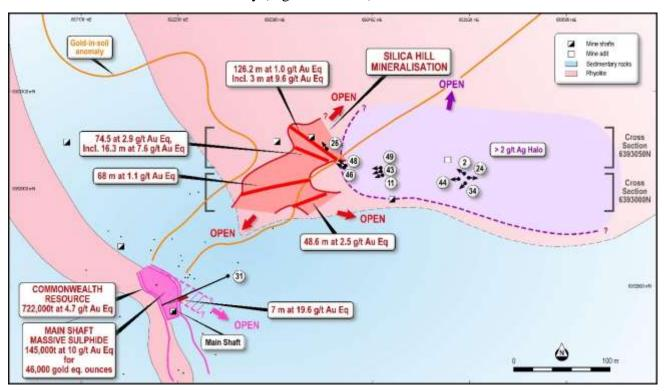
**Figure 3**. Silica Hill: Significant drill results showing new results from CMIPT048 and 049. The mineralisation is open in all directions.
