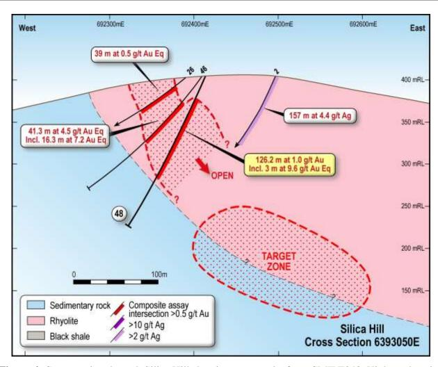
**Figure 4.** Cross section through Silica Hill showing new results from CMIPT048. High grade veins and shoots in CMIPT046 may plunge off section to the south.
