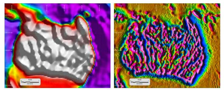
**Figure 1.** Comparison of previous magnetic data (left) and new magnetic data (right) over the Mulga Tank Dunite showing the increased resolution of units within it.
