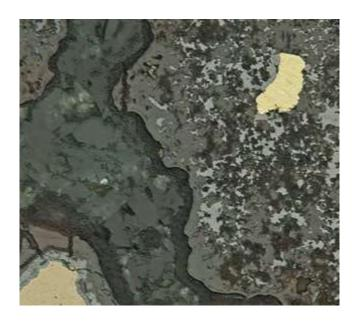
Figure 2. Native gold in top right corner with pyrite (cream) and chalcocite (grey) in bottom left corner. Gold grain is about 50 microns in dimension.
