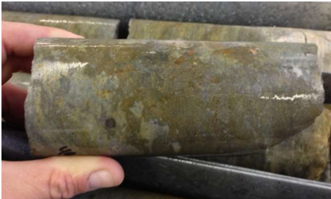
Figure 7: Photograph of diamond drill core from CW27 at 40 m depth. Zones of massive and semi-massive sulphide mineralisation have not been assayed.
