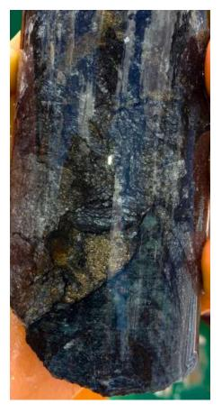
**Figure 2b MTD011.** Clasts of massive nickel sulphide (with copper sulphide) in breccia zone in dunite. The clast may be remobilised from a nearby body of massive sulphide.
