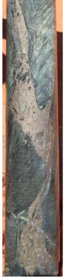
**Figure 2a MTD011.** Disseminated nickel sulphides in adcumulate dunite interpreted to be of magmatic origin. Note all
