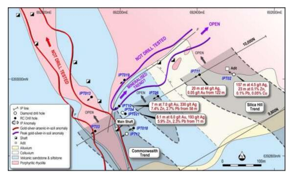
**Figure 3.** Geology and exploration results for the Main Shaft-Silica Hill area. Note the extensive areas of untested soil geochemistry and IP anomalies.
