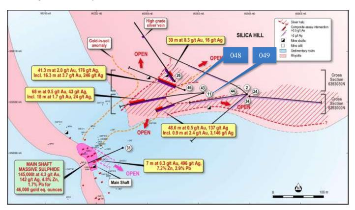
**Figure 2.** Surface geology map showing significant drill intercepts at Silica Hill and Main Shaft and location of CMIPT048 and CMIPT049.
