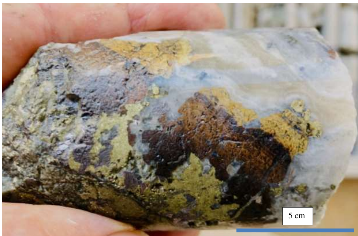
Figure 11. Diamond drill core from 230 metres downhole in RTIPT016. Copper sulphides (chalcopyrite) is yellow coloured at base of core; brown to honey coloured zinc sulphide (sphalerite) in the centre; and colloform to crustiform quartz-chalcedony in upper right.
