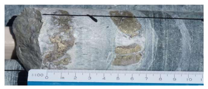
Figure 2. Vein of yellow chalcopyrite (copper) and bronze pentlandite (nickel).
