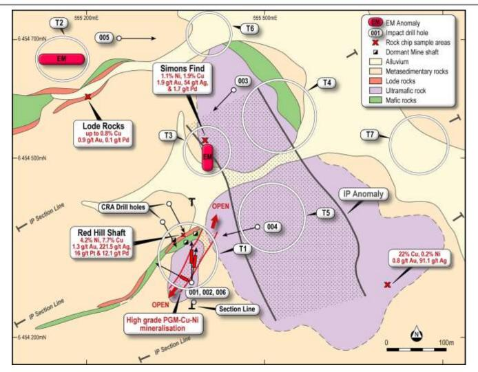
Figure 1. Geology and drill targets (white circles T1 to T7) at the Red Hill Prospect.
