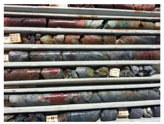
Figure 3. Extensive oxide and sulphide copper-nickel mineralisation, RHDH008.
