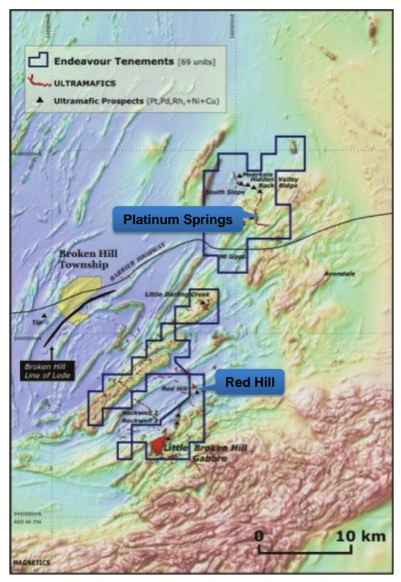
**Figure 3.** Airborne Magnetic image showing the mapped mafic-ultramafic units, joint venture tenements and prospect locations including Red Hill.
