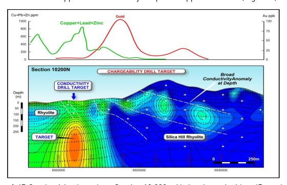
**Figure 4.** IP Conductivity data along Section 10,200 mN showing coincident IP conductivity and lead-zinc-copper-in-soil anomalies. The gold-in-soil anomaly is coincident with strong IP chargeability anomalies (see announcement <u>9 May 2017</u>).
