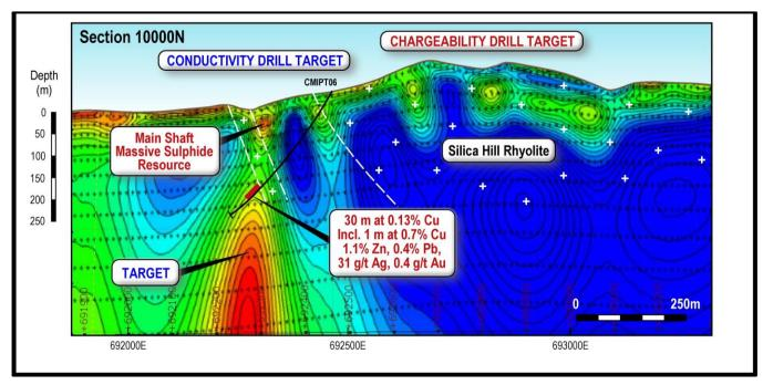
**Figure 3.** IP Conductivity data along Section 10,000 mN showing the massive sulphide body at Main Shaft and copper-rich drill hole CMIPT06.
