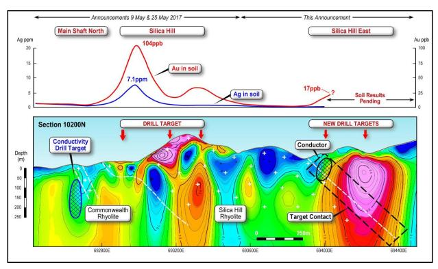
**Figure 6.** Section Line 10,200 mN (Figure 7) showing IP chargeability data from Main Shaft North to Silica Hill East. Note the size and strength of the Silica Hill East anomaly and increasing gold-in-soil response over the target contact and associated conductor.
