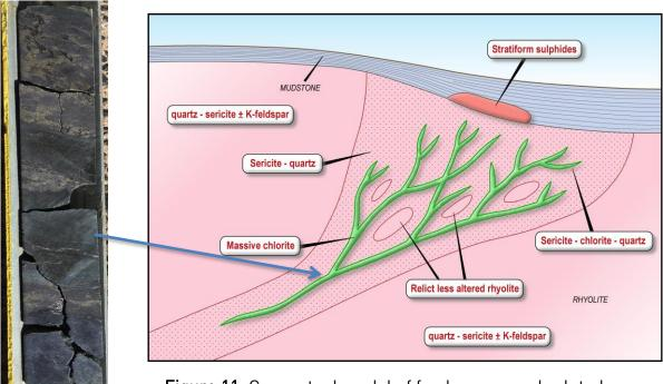
Figure 11. Conceptual model of feeder zone and related massive sulphide from published scientific papers on Eskay Creek. Also shown is drill core and the interpreted position of a "feeder vein" at Silica Hill with strong chlorite (dark green) alteration in the high grade sulphide intercept in CMIPT011 of 0.9 metres at 2.4 g/t gold and 3,146 g/t silver).
