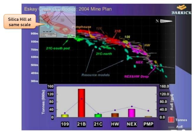
**Figure 10.** Long section of the Eskay Creek gold mine showing the principal ore shoots (eg 21B, NEX etc) coloured by gold equivalent grade. The graph shows the tonnes and gold equivalent grade of each of the shoots. Also shown for comparison at the same scale in the top left hand corner is the cross section of Silica Hill (image is slightly transparent in order to show the upper most Eskay Creek ore shoots).
