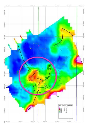
At Little Darling Creek the processed IP data has identified a prominent anomaly close to and in the centre of numerous outcrops of ultramafic rocks that are highly anomalous in nickel, copper and platinum group metals. Several small mine shafts and previous drilling attest to local high grades.
