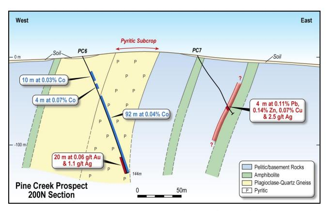
**Figure 15.** Geology and significant drill results of the Pine Creek Project. Note the mineralisation is open at depth.
