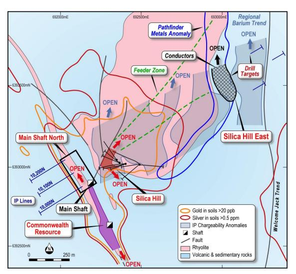
Figure 5. Geology and exploration results for the Silica Hill-Commonwealth area highlighting the new Silica Hill East Prospect on the right hand side of the diagram.
