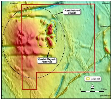
**Figure 3.** Image of regional magnetic data over the Doonia project with warmer colours indicating more magnetic units. A large oval deep-seated anomaly is centred directly under the project area above which a cluster of near surface anomalies is present and interpreted as possible magnetic intrusions. These smaller anomalies are coincident with a gold-bismuth soil geochemistry anomaly (ASX Release 17th November 2020).
