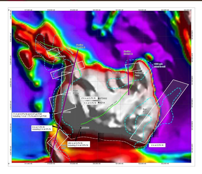
**Figure 2.** Image of the Total Magnetic Intensity from airborne magnetic data over the Mulga Tank Dunite (white outline) showing the modelled geometry of the seven priority EM targets. Note the coincidence with the nickel-in-soil geochemistry and also the location of previous drill hole MTD003 with a best result of 11 m at 0.37% nickel including 1 m at 1.1% nickel that lies immediately south of one of the conductors on the west side of the dunite.
