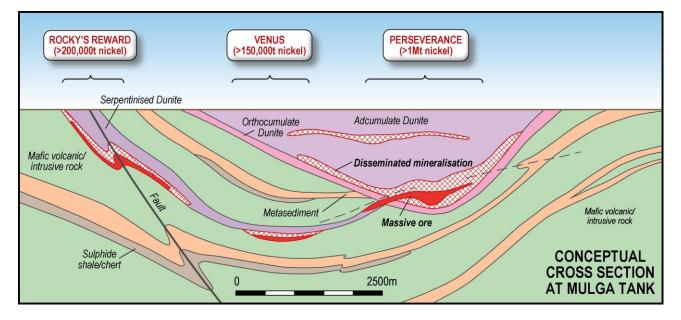
**Figure 4.** Conceptual cross-section for the Mulga Tank Dunite and surrounding area showing the Perseverance and Rocky's Reward exploration model.
