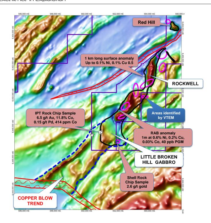
Figure 2. Image of magnetic data over the Rockwell-Little Broken Hill-Copper Blow Trend showing extension of magnetic units along trend from Copper Blow towards the LBHG. Areas identified by VTEM survey shown in pink together with key previous exploration results (see announcement 3<sup>rd</sup> May 2017).
