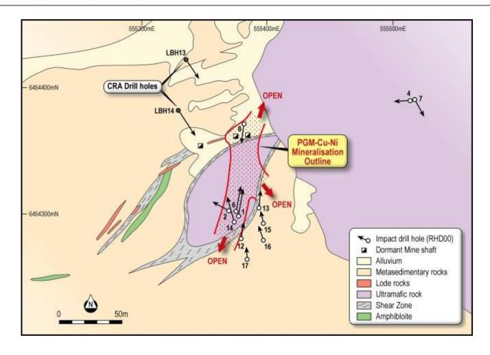
Figure 2. Drill hole location plan for Red Hill (see also Table 2 for drill hole details).
