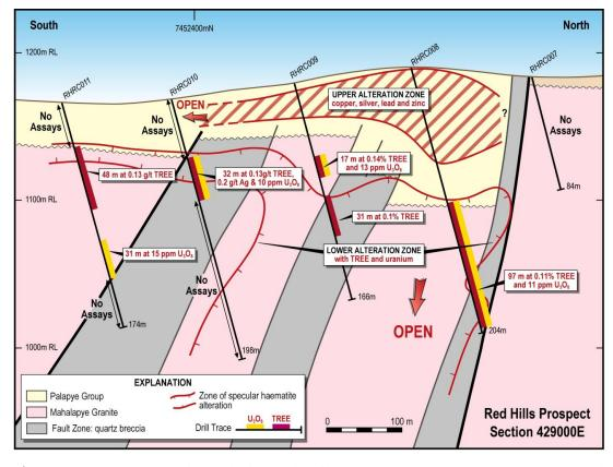
**Figure 5.** Cross section through the Red Hills Prospect on Traverse 429,000 mE and showing the Upper Zone and Lower Zone of the alteration system.
