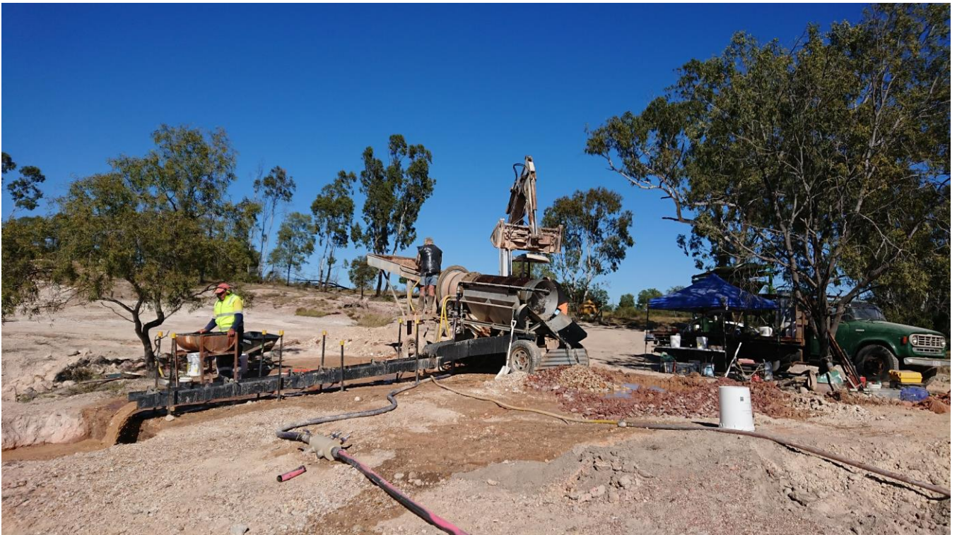
Figure 6. Wet processing plant set up at Blackridge. A small trommel is fed from a hand apron with oversize material exiting from the right and dense and fine material falling through the screen of the trommel into the black sluice.
