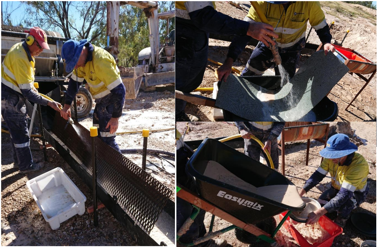
Figure 7. Process of extracting gold from the sluice to produce a panned concentrate.
