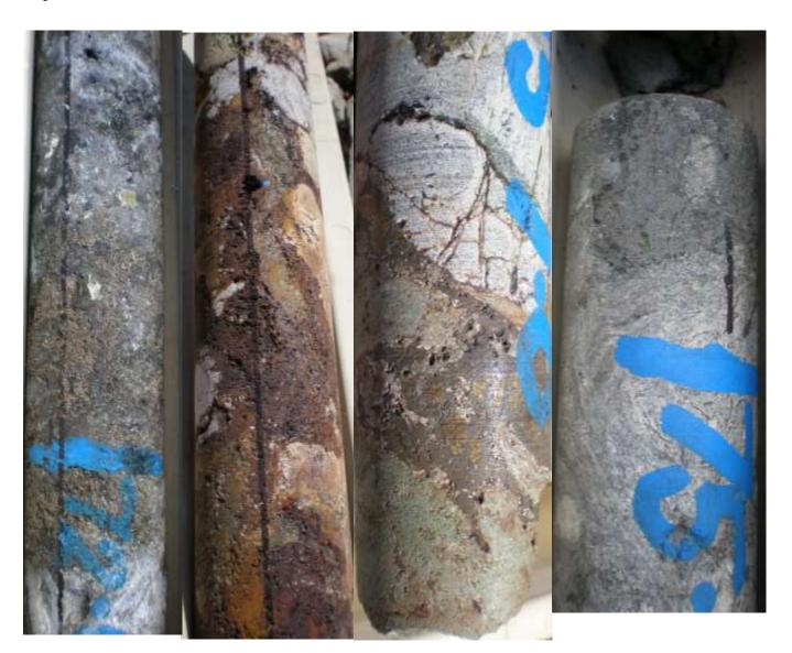
Figure 2a. Nickel and iron sulphides.
