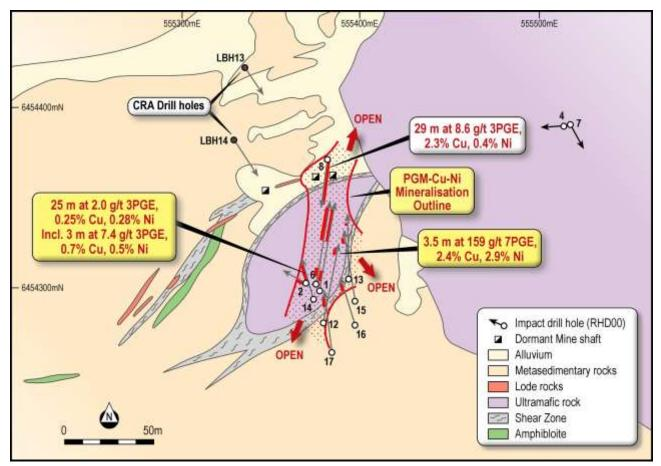
**Figure 1.** Geology and drill hole locations at Red Hill showing the three significant assays of the current drill programme in holes RHD008, 012 and 014. Also shown in red are significant assays or zones of mineralisation identified from logging. Assays are awaited for Holes 013, 015, 016 and 017.
