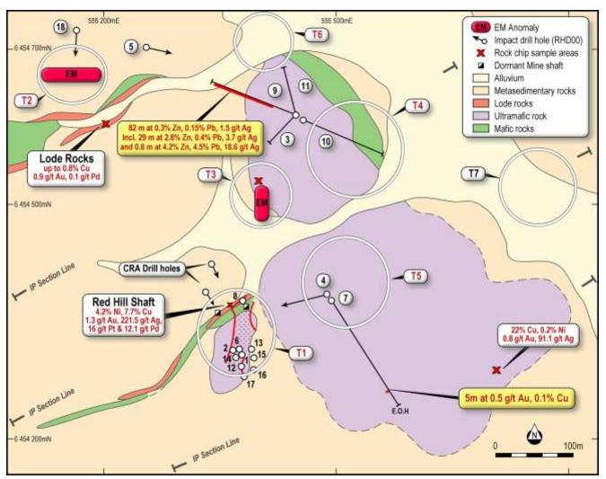
Figure 2. Geology and drill hole locations in the greater Red Hill area showing significant assays in Holes RHD007 and 009. Note that the intercepts are projected to surface and mineralisation occurs predominantly at the base of or below the ultramafic intrusion.
