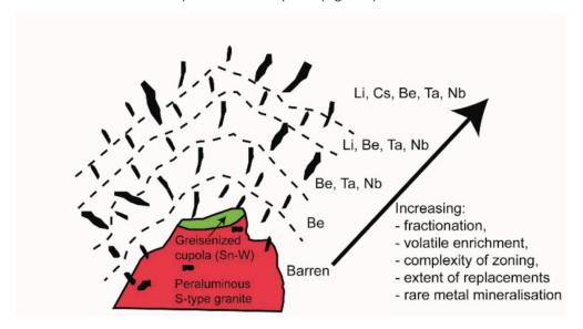
**Figure 8**. Cartoon of a widely used exploration model for zoned pegmatite systems showing a core of beryllium (Be) dominant mineralisation passing outwards to tantalum, niobium, lithium and caesium dominant mineralisation.
