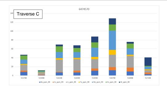
**Figure 7.** Stacked bar charts of additive response ratios for Traverse C. The elements are plotted in order from bottom to top as per the exploration model and suggest they may be part of a zoned system (Figure 7).
