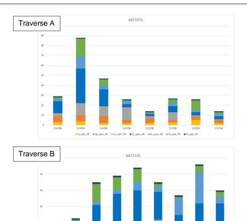
Figure 3. Stacked bar charts of additive response ratios for Traverse A (top) and Traverse B (bottom).
