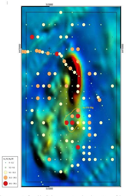
**Figure 5.** Combined response ratios for gold-palladium-magnesium plotted on an image of the regional magnetic data (more magnetic units in warmer colours) and showing a coherent anomaly about 500 metres in diameter. The elevated magnesium responses show a strong correlation to elevated REE responses. This area has not been field checked.
