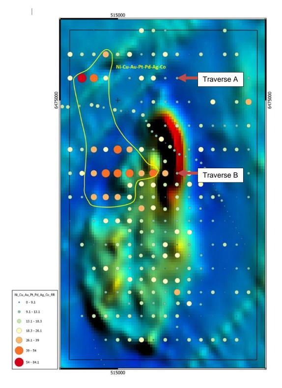
**Figure 2.** Combined response ratios for nickel-copper-cobalt-platinum-palladium-silver-gold-cobalt plotted on an image of the regional magnetic data (more magnetic units in warmer colours). The main soil anomaly is highlighted and is mostly coincident with rocks of low magnetic response and interpreted as part of a large mafic intrusion. The strong magnetic unit in the northeast is probably a unit of banded iron formation.
