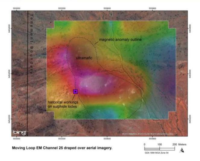
Figure 7. Image of mid-to late time channel EM data from the Red Hill Prospect. The red-to-white colour indicates areas of higher conductivity.
