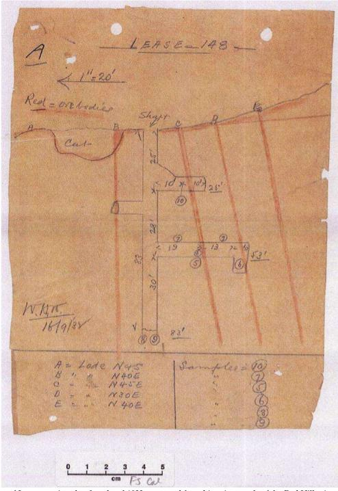
Figure 8. One of 3 cross section sketches dated 1932 recovered from historic records of the Red Hill mine showing the location of the four lodes and the main shaft.
