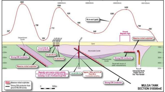
**Figure 5.** Section line 518500 mE showing the interpreted ultramafic rocks, the West Plate conductors (north), South Plate conductor (south), nickel-in-soil values highlight drill results and interpreted massive nickel sulphide drill targets.
