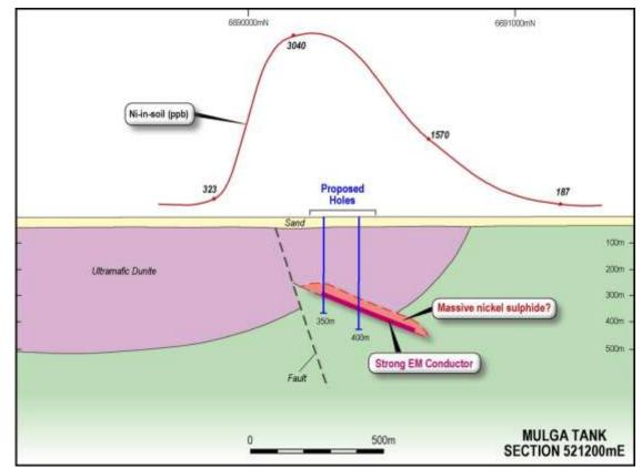
Figure 4. Section line 521200 mE showing the interpreted ultramafic rocks, the Northeast Plate conductor, nickel-in-soil values, interpreted massive nickel sulphide and planned drill holes.
