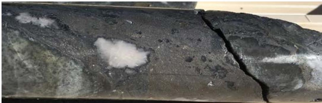
**Figure 4.** High grade “feeder vein” at 114.5 metres depth in Hole 63 containing silver, zinc, lead and copper with accessory molybdenum, antimony, tin and bismuth.
