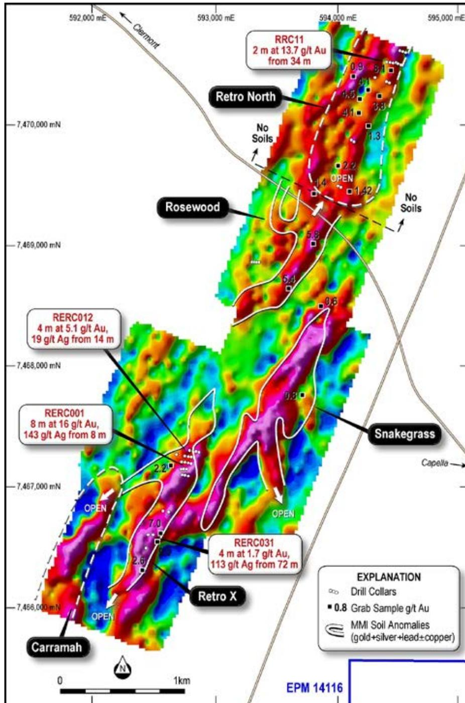
**Figure 12.** Image showing the resistivity results of the gradient array IP survey at Clermont. The warmer colours are areas of high resistivity and are likely to be quartz veins. Also shown are the five drill targets and previous relevant drill results.
