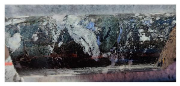
**Figure 2.** Large "slugs" of grey-blue molybdenite in a zone of fractured quartz veins with associated biotite (dark brown) and chlorite (green).
