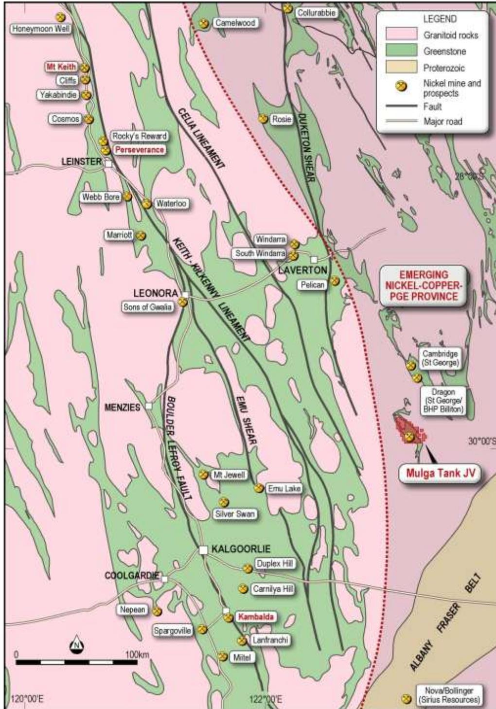
**Figure 1.** Location of Impact’s Mulga Tank Project and significant nickel sulphide mines and prospects including Perseverance and Rocky’s Reward deposits with new nickel-copper-PGE discoveries in the emerging nickel-copper province to the east.
