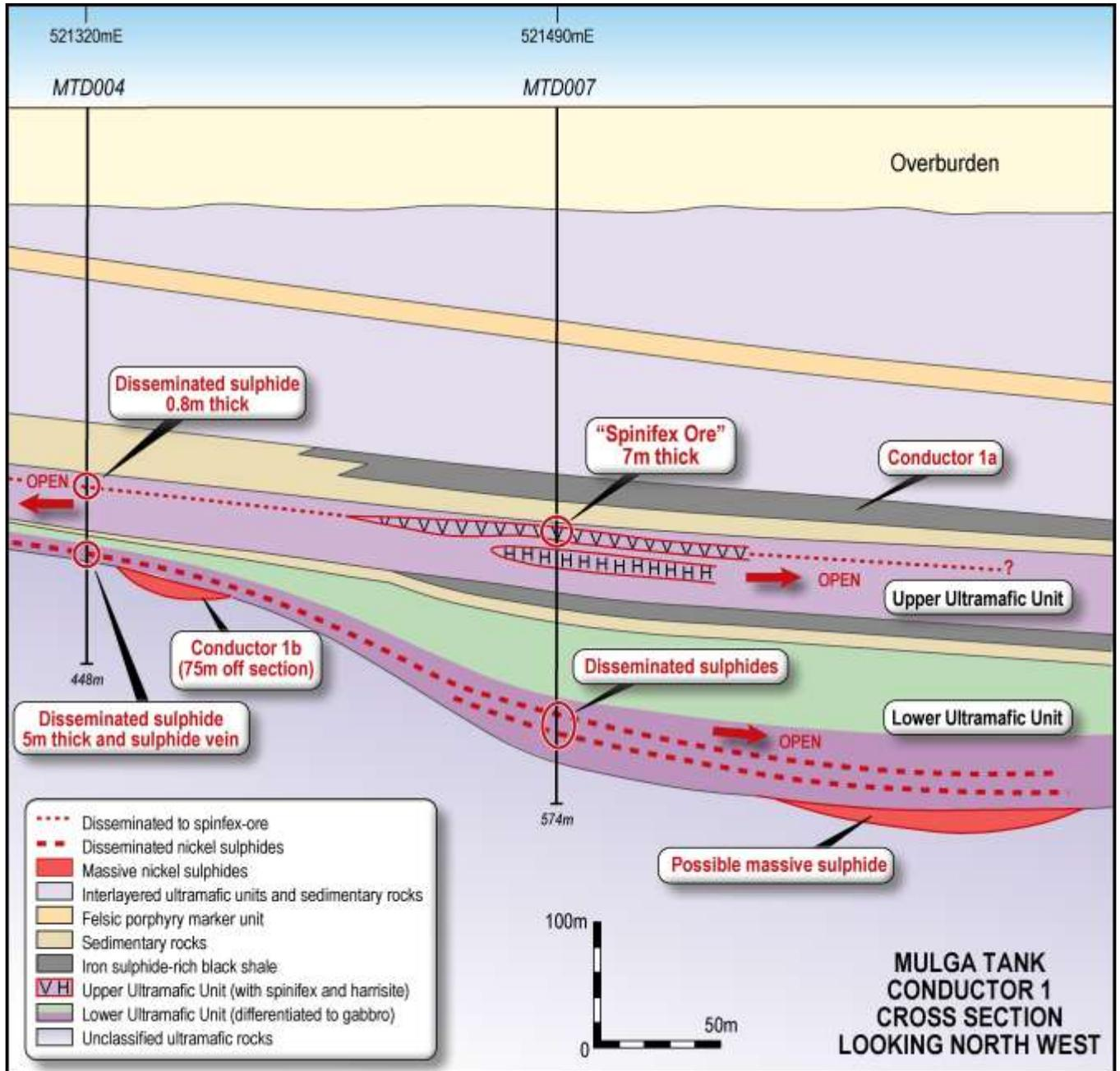
Figure 5. Interpreted cross section looking north west, Conductor 1.
